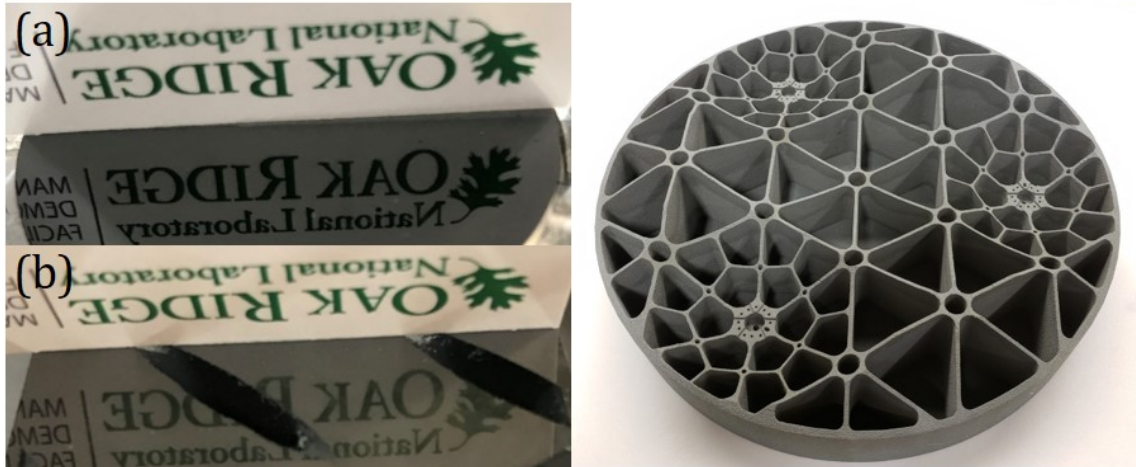
Figure 3.8: (a) Finish ground CVD SiC surface. (b) Finish ground AM SiC surface. (c) A 270 mm diameter light weighted mirror blank manufactured by AM process.
