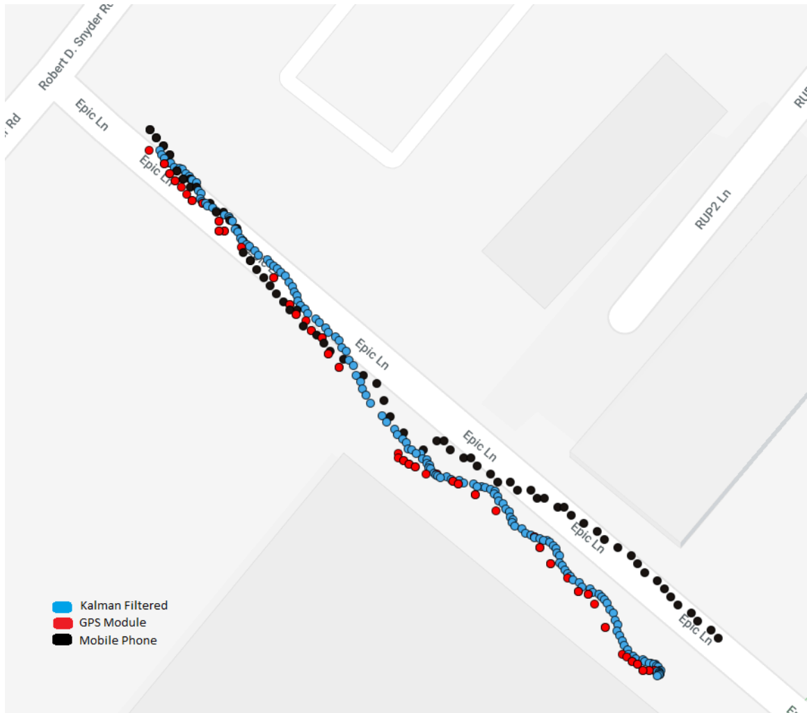
Figure 5.16: Results obtained from the system when GPS was manually switched off.
