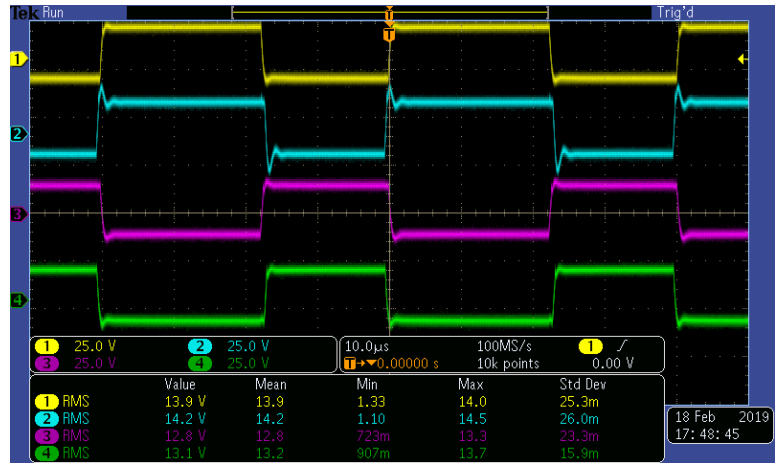
Figure 7-34: Gate Drive switching signals for duty ratio of 0.55
