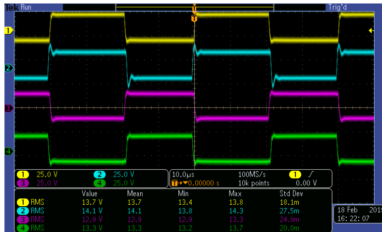
Figure 7-28: Output current for V_{out} = 29\text{ V} , V_{in}=35\text{V} , D=0.45
