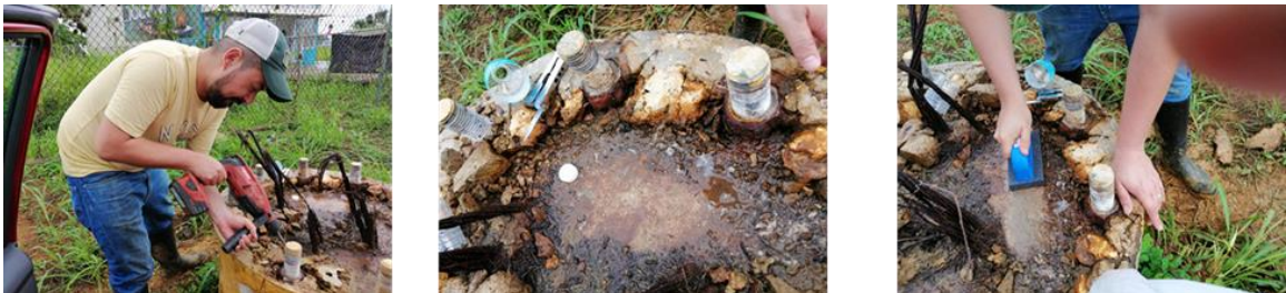
Figure 6-10: Drilled shaft location of the PIT test
