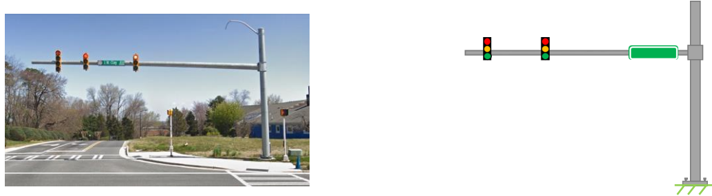
b. Photo of a mast arm structure (MATS) and its schematic representation
