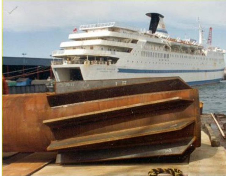
Figure 4-16: Photo of SPINFIN finned pipe pile (Image from PND Engineers).
