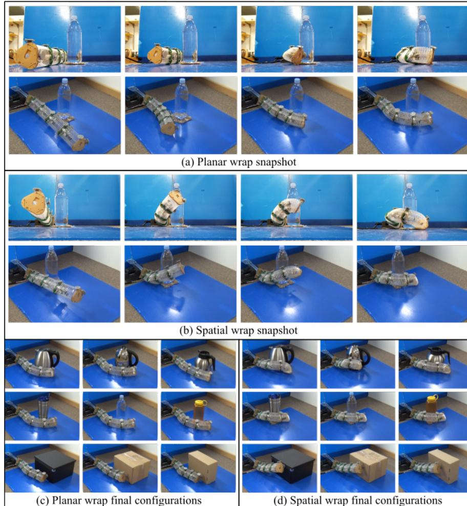
Figure 32: The motion snapshots of (a) planar and (b) spatial continuum wraps around the bottle, where the top and bottom rows show the motion of the same wrap from two view angles respectively, (c) final configurations for the remaining objects with planar wraps, (d) spatial wrap final configurations.
