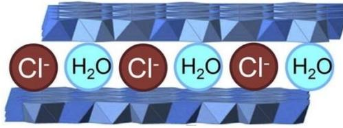
Figure 1.3. Schematic representation of Friedel's salt structure (Li et al. 2017)
