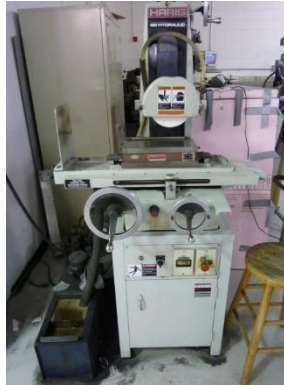
Figure D.1. Bridgeport Harig 612 surface grinder used to cut the silicon pieces into secondary interferometers.
