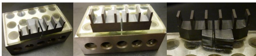
Figure D.14. Additional images of the part after cutting in half to yield two interferometers.
