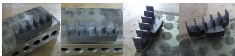
Figure D.13. Additional images following the final cuts that produce the blades before the final cut that separates the part into two interferometers.
