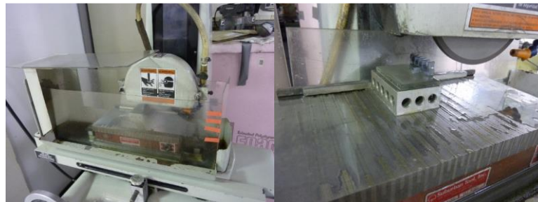
Figure D.4. Surface grinder with clear plastic shielding to contain the flood coolant.
