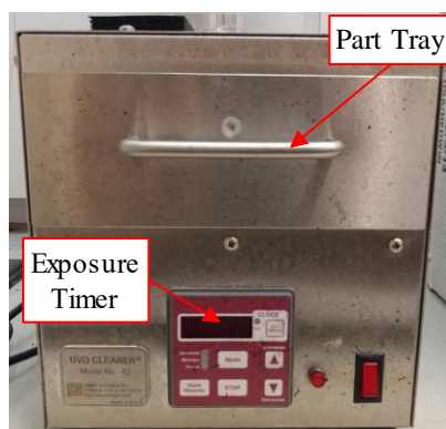
Figure 4.25. UVO-Cleaner Model 42 used to cure the UV epoxy.
