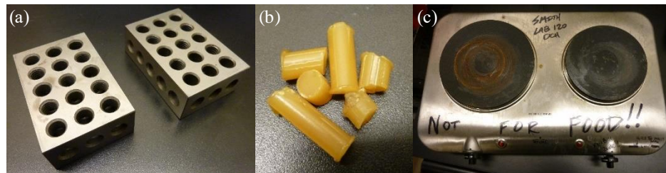
Figure D.2. Components shown are (a) 1-2-3 blocks, (b) optical wax, (c) and the hot plate necessary for mounting and securing silicon piece to be machined.
