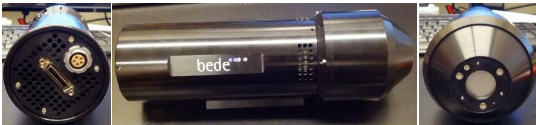
Figure 3.13. The branded Photonic Science camera that used a scintillator coated fiber banded directly bonded to the CCD.
