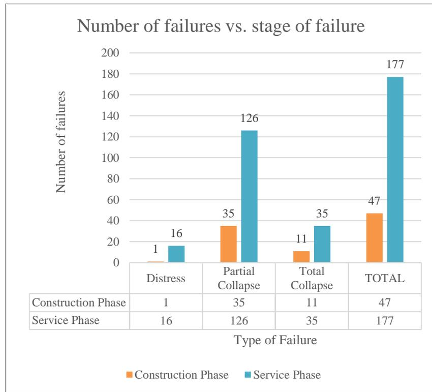
Figure 2: Number of failures against stage of failure
