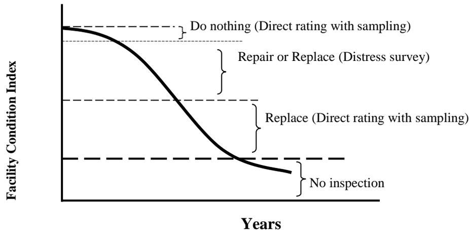
Figure 5: Life cycle repair vs replacement needs adapted from Uzarski (2007)
