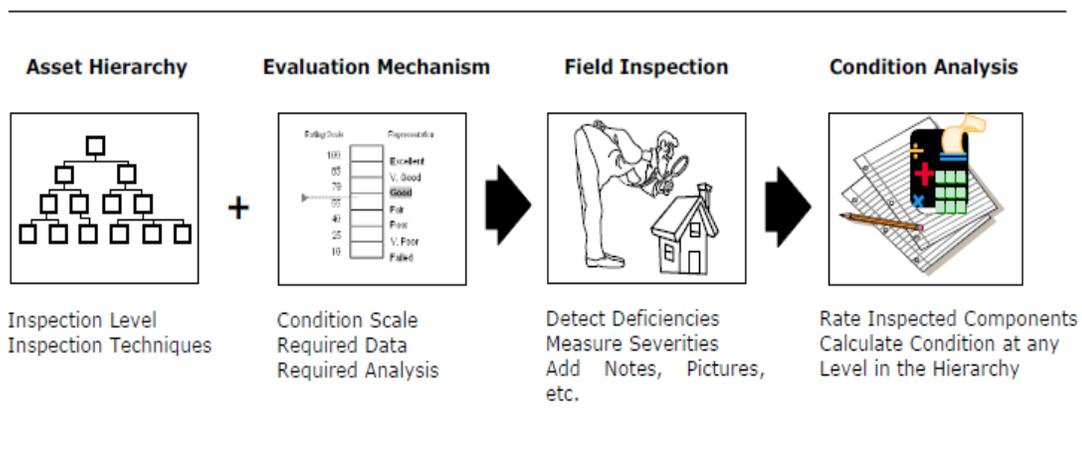
Figure 4: Main Steps in FCA adapted from Lavy et al. (2001)
