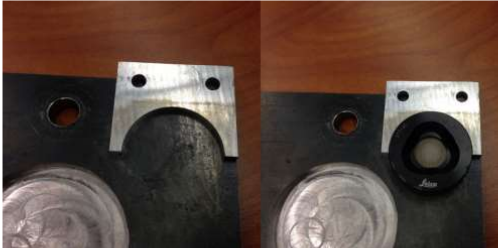
Figure 7: Fixture used for placing SMR nest 1 & 2 on PS4.
