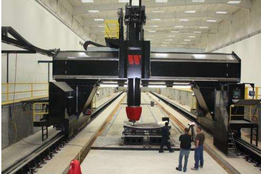
Figure 1: Largest five-axis gantry mill in North America built by Ingersoll Machine Tools. (28 feet wide, 240 feet long, 10 feet under the gantry) [2].
