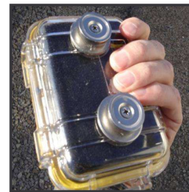
Figure 6.14.b: The box and its magnets. All parts of the temperature sensing are enclosed inside the magnet. (The photo shows one of the temperature sensing nodes that were deployed in Paradise substation, KY).
