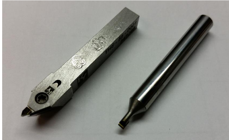
Figure 3.3: (left) Insert-style turning tool, (right) square SCD endmill.
