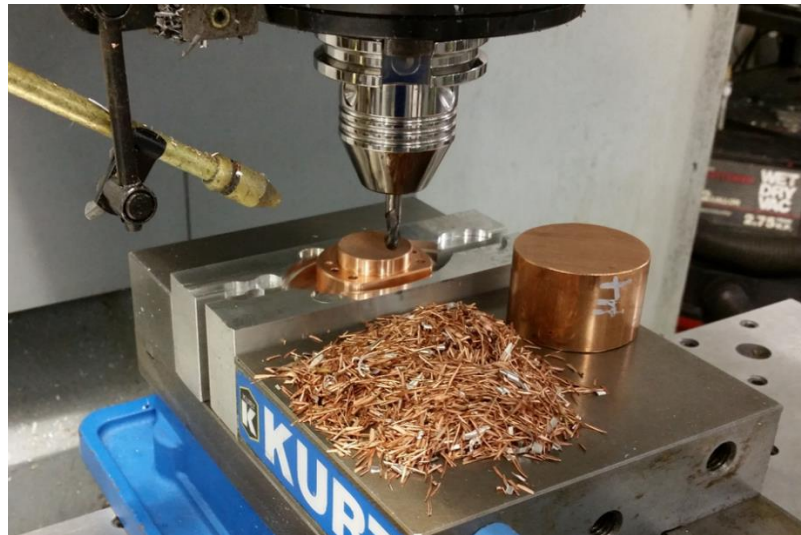
Figure 8.4: Primary mirror conventional CNC machining. Clockwise from center: machined component, raw bar stock blank, resulting chips.
