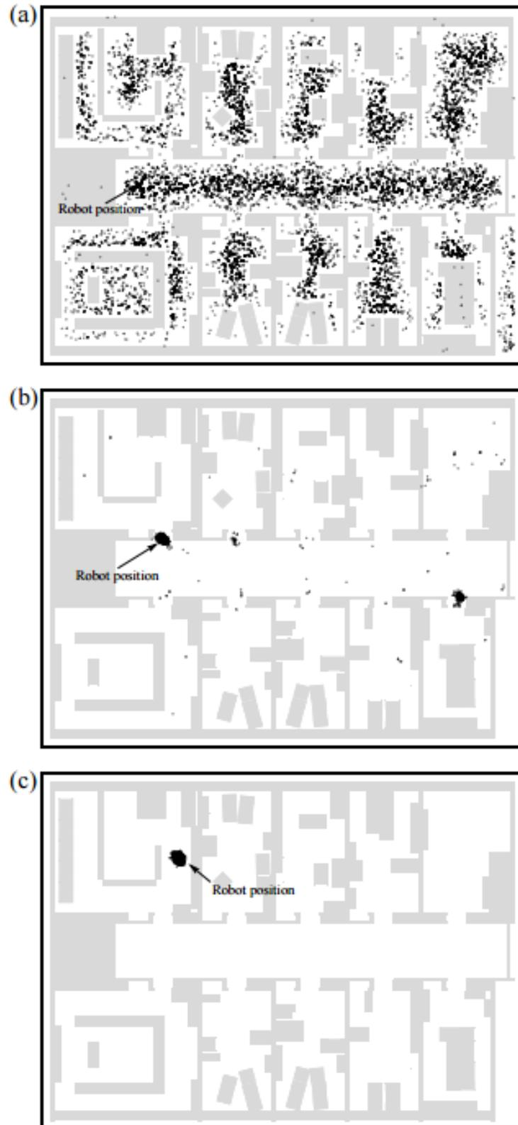
Figure 5.1: Particle filter for mobile robot localization [7].
