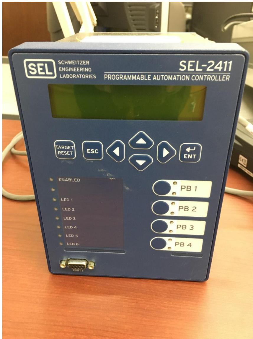
Figure 49: Programmable Automation Controller SEL - 2411
