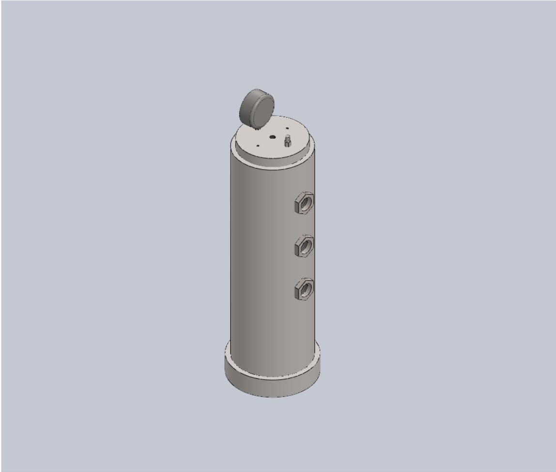
Figure 38: Plain Carbon Steel Pressure Chamber Model
