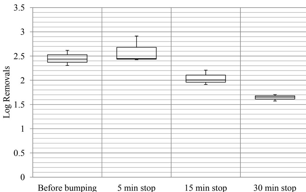
Figure 4.59 *Cryptosporidium*-sized Microsphere Removals by DE Filtration Before and After Filter Bumping with a 5-minute, 15-minute, and 30-minute Filter Stops (number of microsphere seeding cycles = 3), 0.7 kg·DE/m<sup>2</sup>, Filtration Rate of 3.6 m/h (number of experiments = 2, number of samples = 3)
