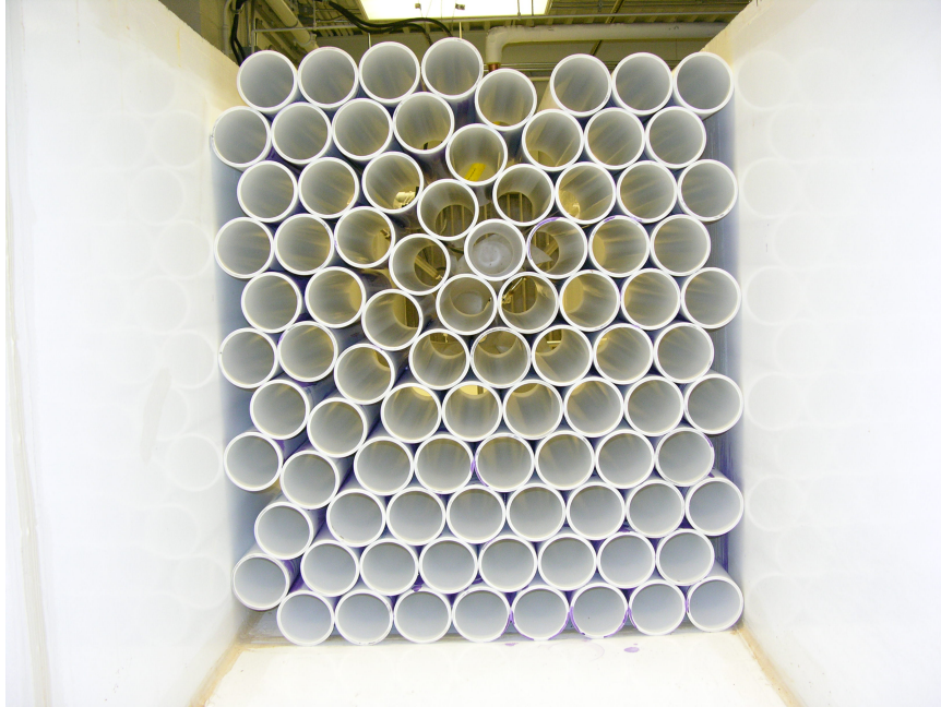
Figure 2.13: PVC flow straightener immediately downstream of pump.
