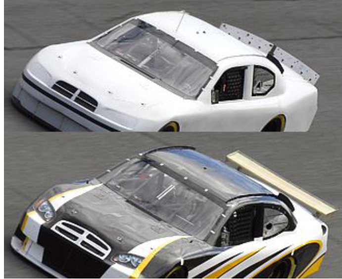
Figure 4.2: Image of the COT fitted with a spoiler (top) and wing (bottom). From [110].
