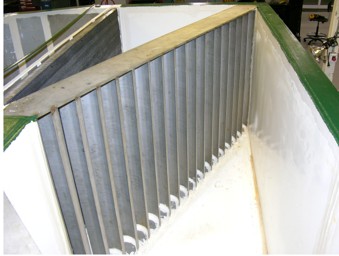
Figure 2.12: View of turning vanes entering the nozzle section of the channel.
