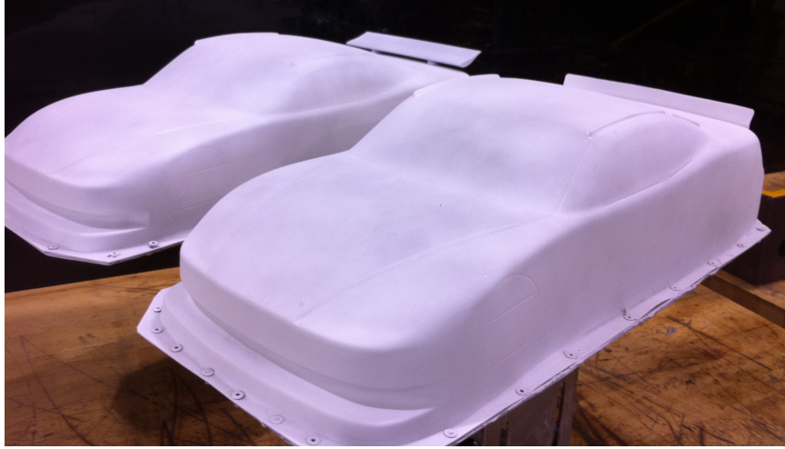
Figure 4.3: 10% scale models of COT with wing (back) and spoiler (front). The models are translucent, thermoformed polycarbonate, but a temporary powder coating is applied for the photograph.
