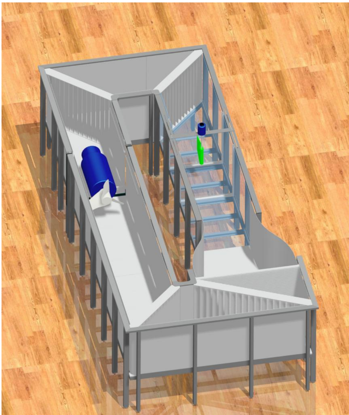
Figure 2.3: Recirculating water channel rendering. Flow is counterclockwise.
