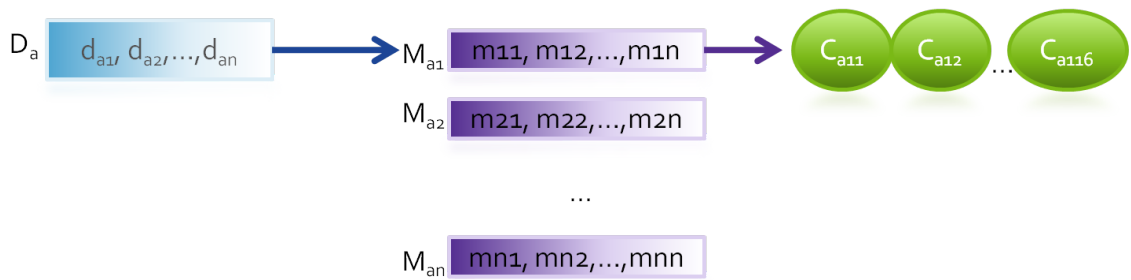
Figure 14: A visualization of the data stored for a user a , where D is the set of answers the user submitted for the first part of the questionnaire, M_{a1}-M_{an} is the set of mood vectors for that user, and C is the set of classifiers for each mood vector ( M_{a1} , in the case of the above figure)
