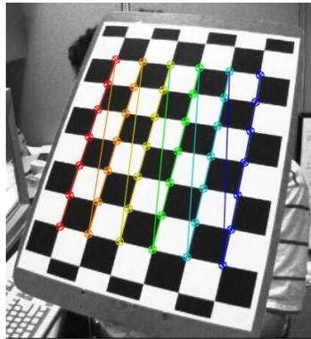
Figure 2.2: A checkerboard pattern used for camera calibration. [1]
