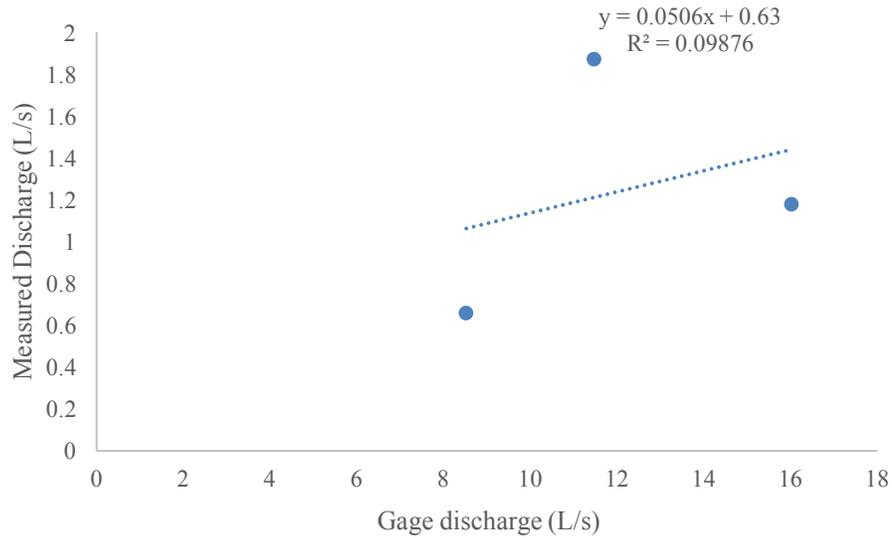
C2 Concurrent flow approach between R1 gage discharge and field measured discharge, regression formula and  $R^2$ .
