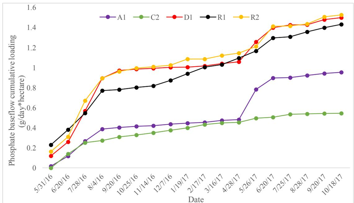
Figure 34. Monthly concurrent flow phosphate baseflow cumulative loading (g/day\*hectare) over time. Agricultural outlet in purple, control in green, developed outlet in red, R2 mainstem in yellow, and the watershed loading (R1) in black.
