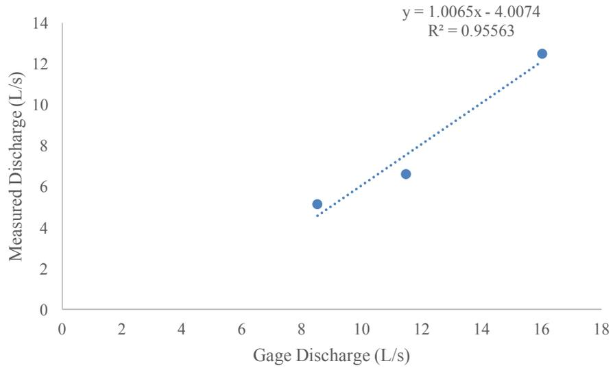
R2 Concurrent flow approach between R1 gage discharge and field measured discharge, regression formula and  $R^2$ .
