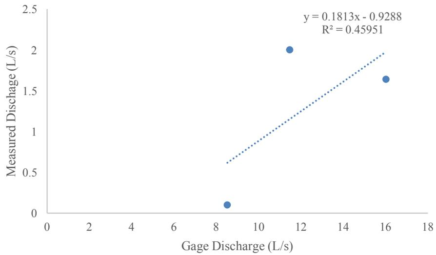
D1 Concurrent flow approach between R1 gage discharge and field measured discharge, regression formula and  $R^2$ .
