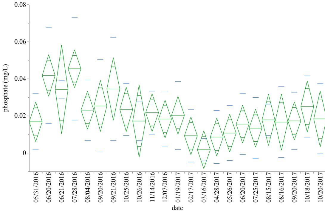
Figure 19. Mean phosphate concentration in mg/L averaged across all sites over time, showing mean error (green diamonds) and standard deviation (blue bars).
