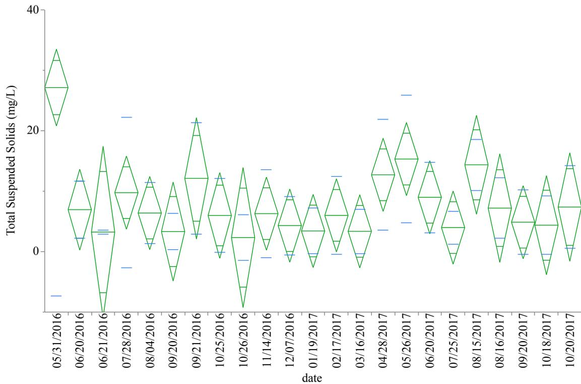
Figure 26. Mean TSS concentration in mg/L averaged across all sites over time, showing mean error (green diamonds) and standard deviation (blue bars).
