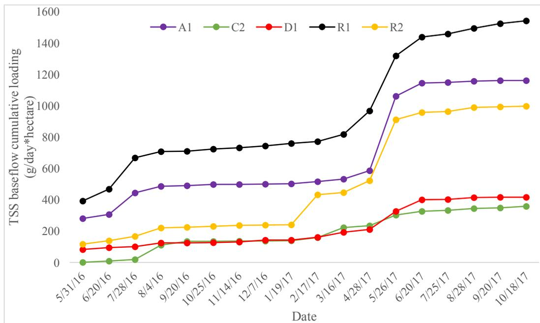
Figure 36. Monthly concurrent flow TSS baseflow cumulative loading (g/day\*hectare) over time. Agricultural outlet in purple, control in green, developed outlet in red, R2 mainstem in yellow, and the watershed loading (R1) in black.
