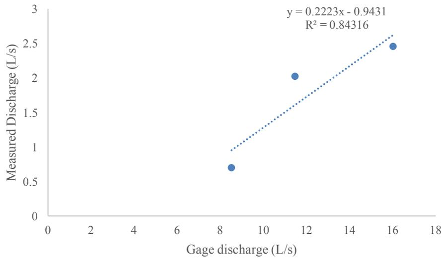
A1 Concurrent flow approach between R1 gage discharge and field measured discharge, regression formula and  $R^2$ .
