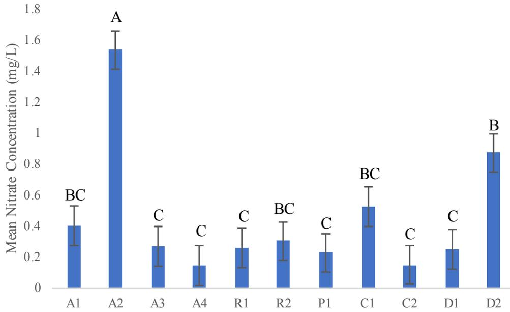
Figure 24. All pairs Tukey HSD mean comparison between all sites for nitrate concentration. A represents a mean that is significant from B which is significant from C. BC represents sites that are not significantly different from each other, B, or C. The sample number for each site N=18 except for A2 and C2 for which N=17.
