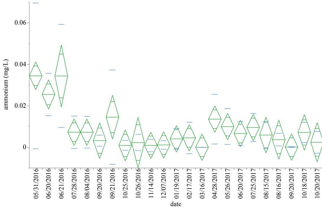
Figure 16. Mean ammonium concentration in mg/L averaged across all sites over time, showing mean error (green diamonds) and standard deviation (blue bars).
