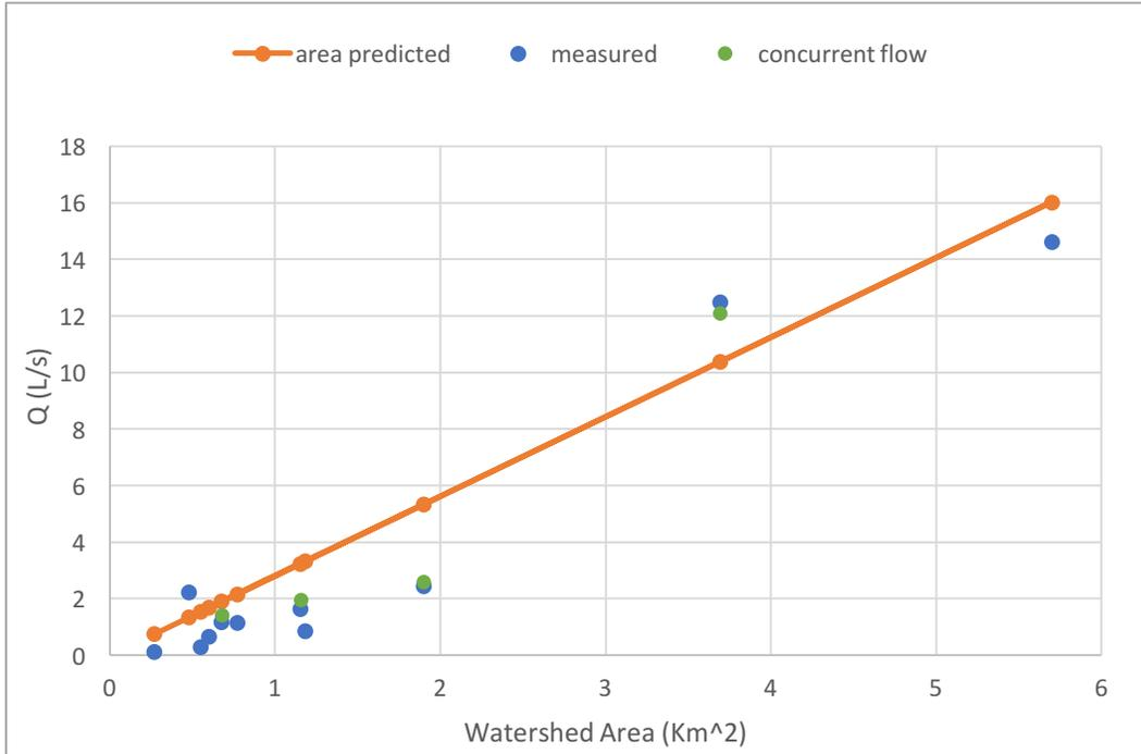
Figure 12. Relationship between watershed area and discharge for 9/20/17. Blue shows the measured discharge for each site based on the corresponding watershed area. Orange shows the drainage area ratio approximation and green shows the concurrent flow approximation.
