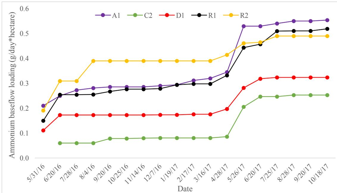
Figure 33. Monthly concurrent flow ammonium baseflow cumulative loading (g/day\*hectare) over time. Agricultural outlet in purple, control in green, developed outlet in red, R2 mainstem in yellow, and the watershed loading (R1) in black.
