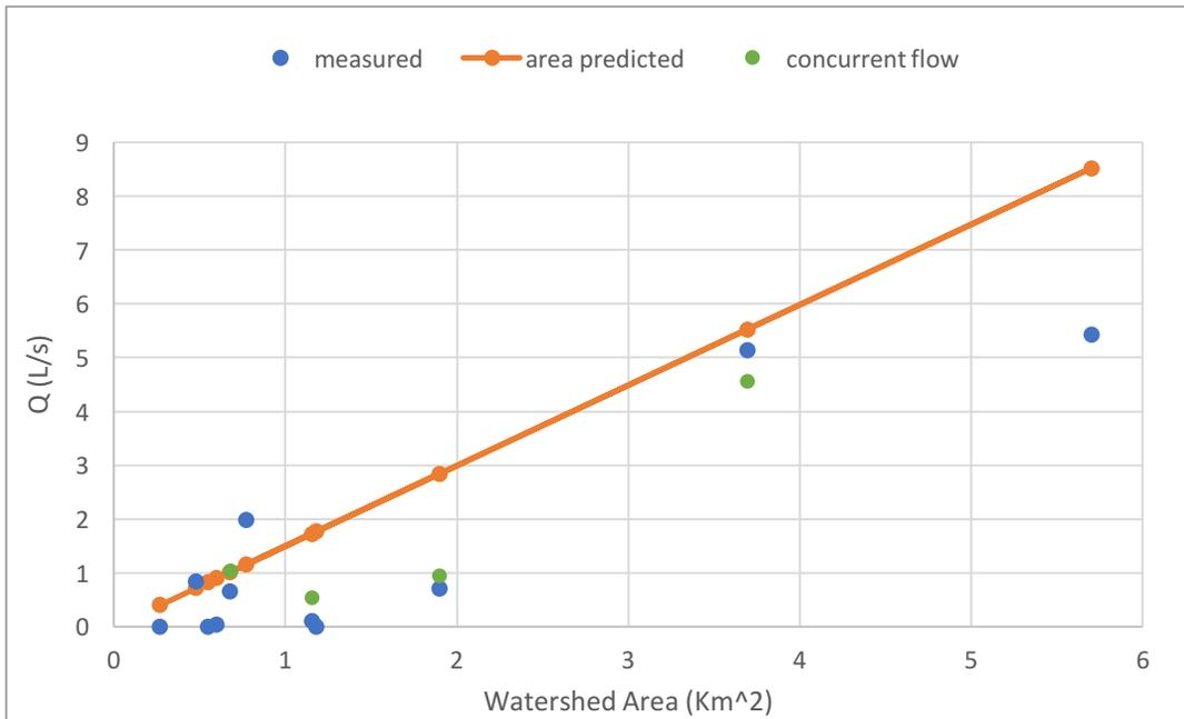
Figure 13. Relationship between watershed area and discharge for 10/18/17. Blue shows the measured discharge for each site based on the corresponding watershed area. Orange shows the drainage area ratio approximation and green shows the concurrent flow approximation.
