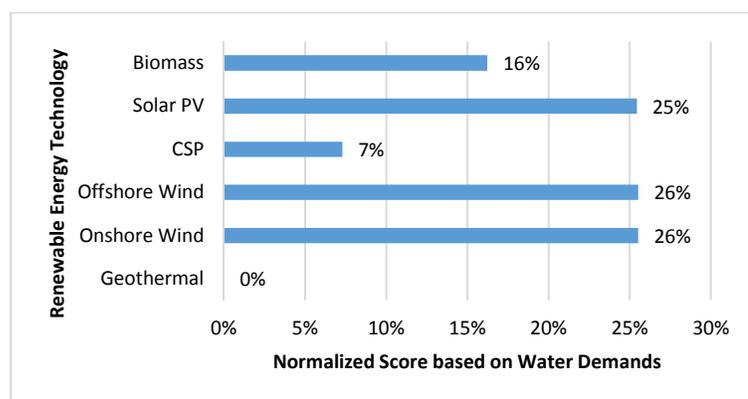
Figure 4-14: Normalized Scores based on Water Demand
