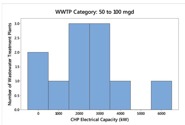
Figure 6-7: Histogram of WWTP CHP Electrical Capacities for WWTP with Average Flows of 50 to 100 Mgd
