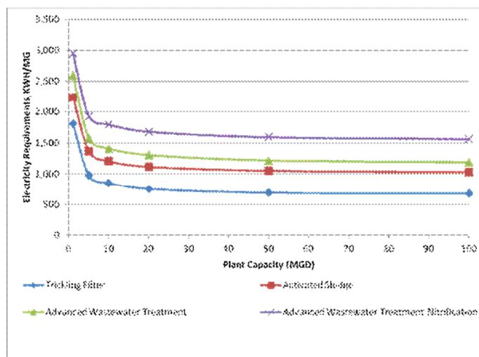
Figure 6-1 Electricity Demand for Wastewater Treatment by Size of Plant and Treatment Type Source: EPRI (2002)
