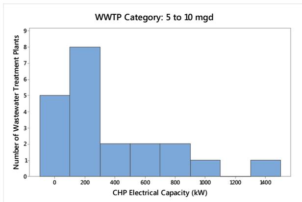
Figure 6-4: Histogram of WWTP CHP Electrical Capacities for WWTP with Average Flows of 5 to 10 Mgd
