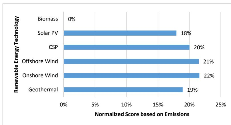
Figure 4-11: Normalized Scores based on Emissions
