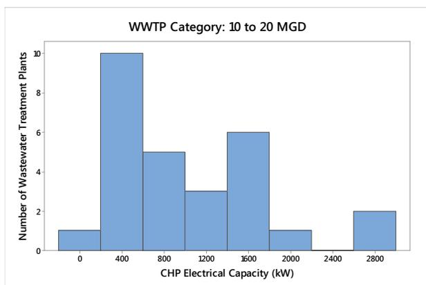
Figure 6-5: Histogram of WWTP CHP Electrical Capacities for WWTP with Average Flows of 10 to 20 Mgd
