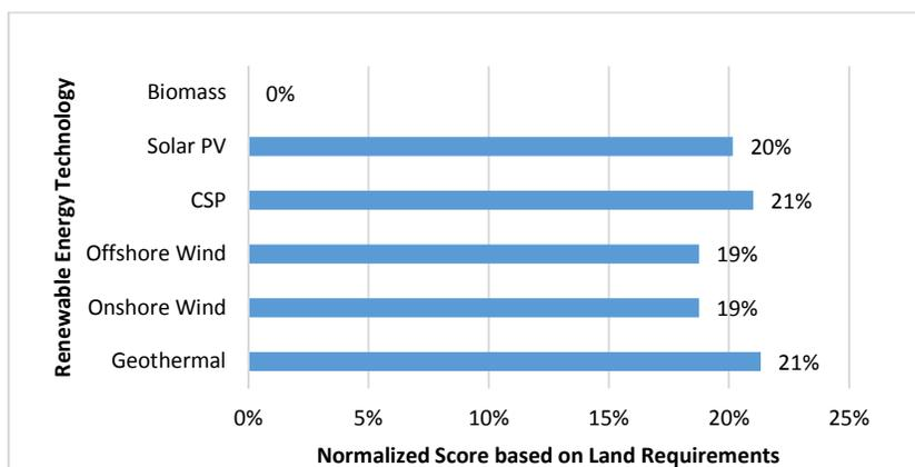
Figure 4-12: Normalized Scores based on Land Requirements
