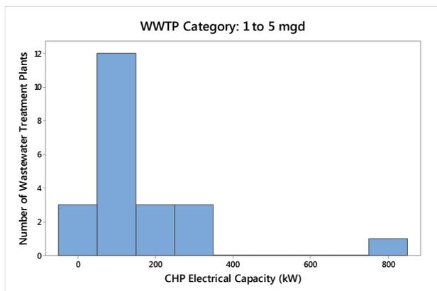
Figure 6-3: Histogram of WWTP CHP Electrical Capacities for WWTPs with Average Flows of 1 to 5 Mgd
