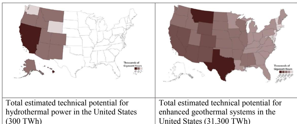
Figure 4-18: Hydrothermal and EGS Technical Potential Comparison
