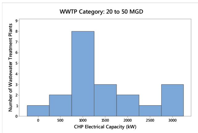
Figure 6-6: Histogram of WWTP CHP Electrical Capacities for WWTP with Average Flows of 20 to 50 Mgd
