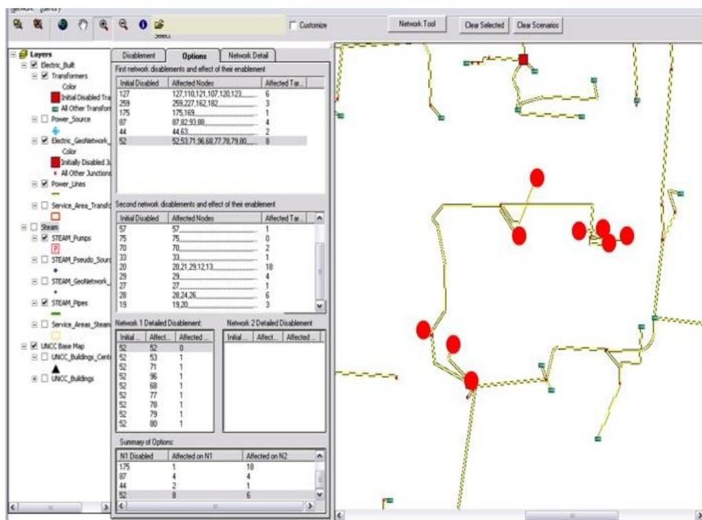
FIGURE 17: On screen outage simulation with CIE
