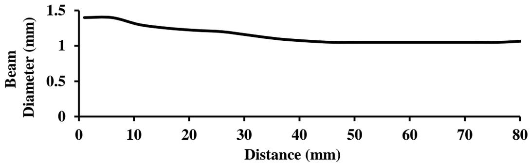
Figure 2.8: Beam diameter as a function of working distance for the flat-top probe with a 9  $\mu\text{m}$  core diameter optical fibers. The beam remains at approximately 1 mm diameter over a distance of 40 - 80 mm.
