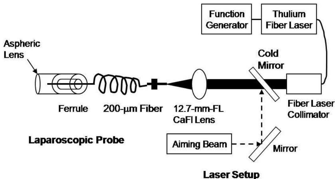
Figure 3.4: Diagram of experimental setup with fiber optic assembly for the laparoscopic laser probe (left) and laser equipment (right).
