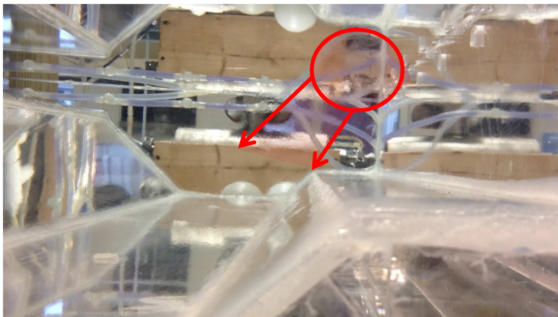
Figure 3.13: Visible density current in initial dosing
