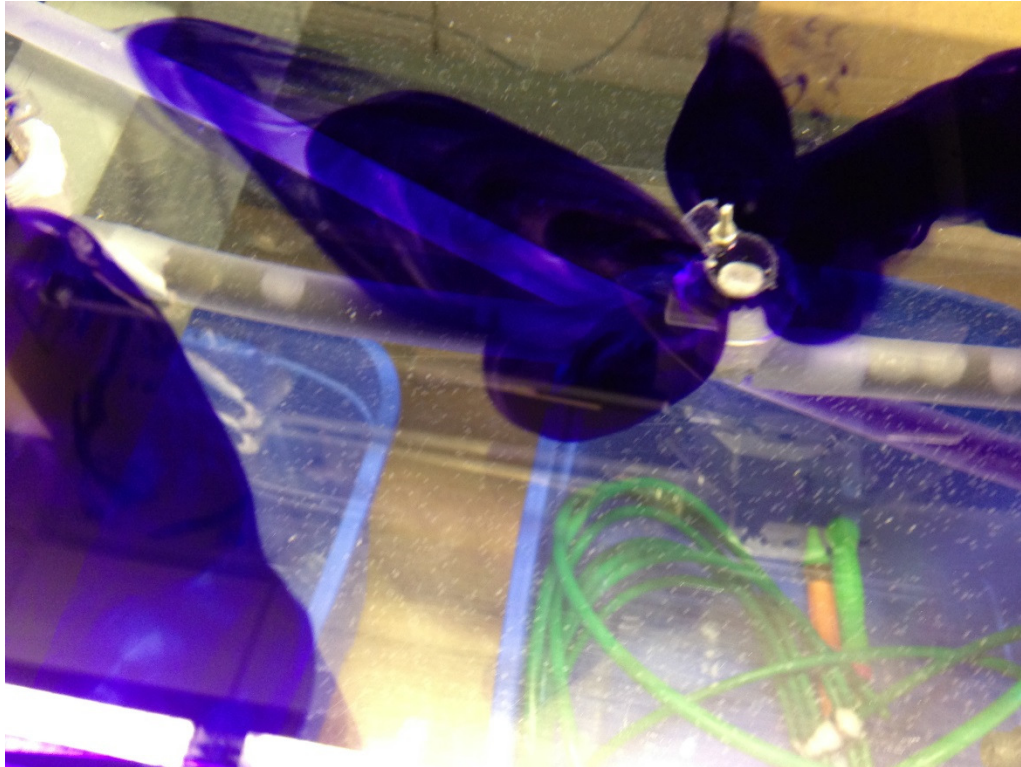
Figure 4.31: Dye exiting bottom mounted inlet t = 17 seconds
