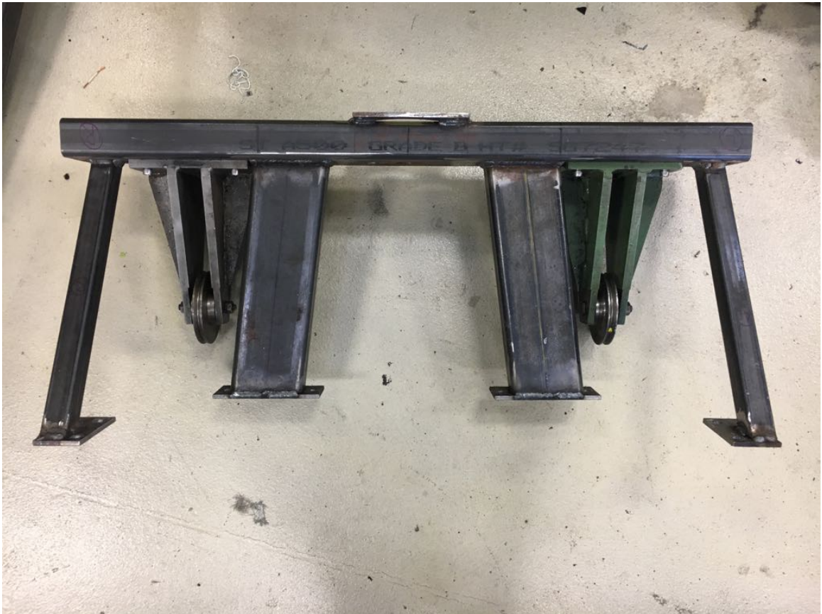
Figure 3.5: Fixture Frame for rear carriage mounting.
