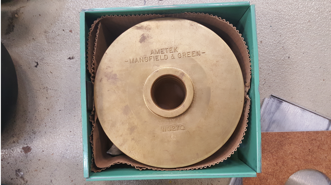
Figure 2.2: Dead Weights used for calibrating reference load cell.
