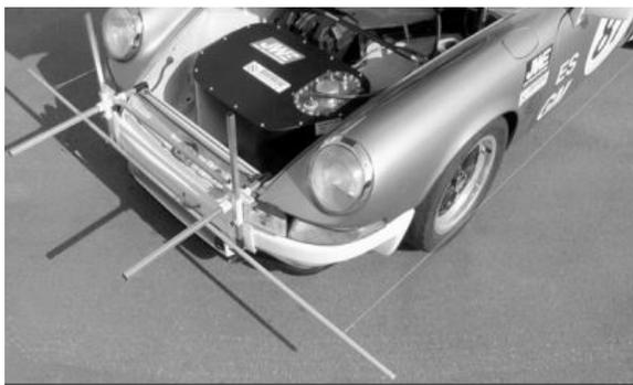
Figure 2.18: Toe alignment using strings [29].
