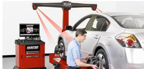
(b) Externally referenced measurement systems.
