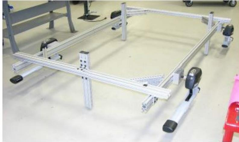
Figure 3.20: Aluminum alignment head test fixture.
