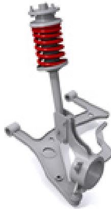
Figure 2.2: MacPherson Strut suspension [6].
