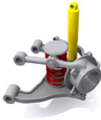
Figure 2.4: Multi-link suspension [6].
