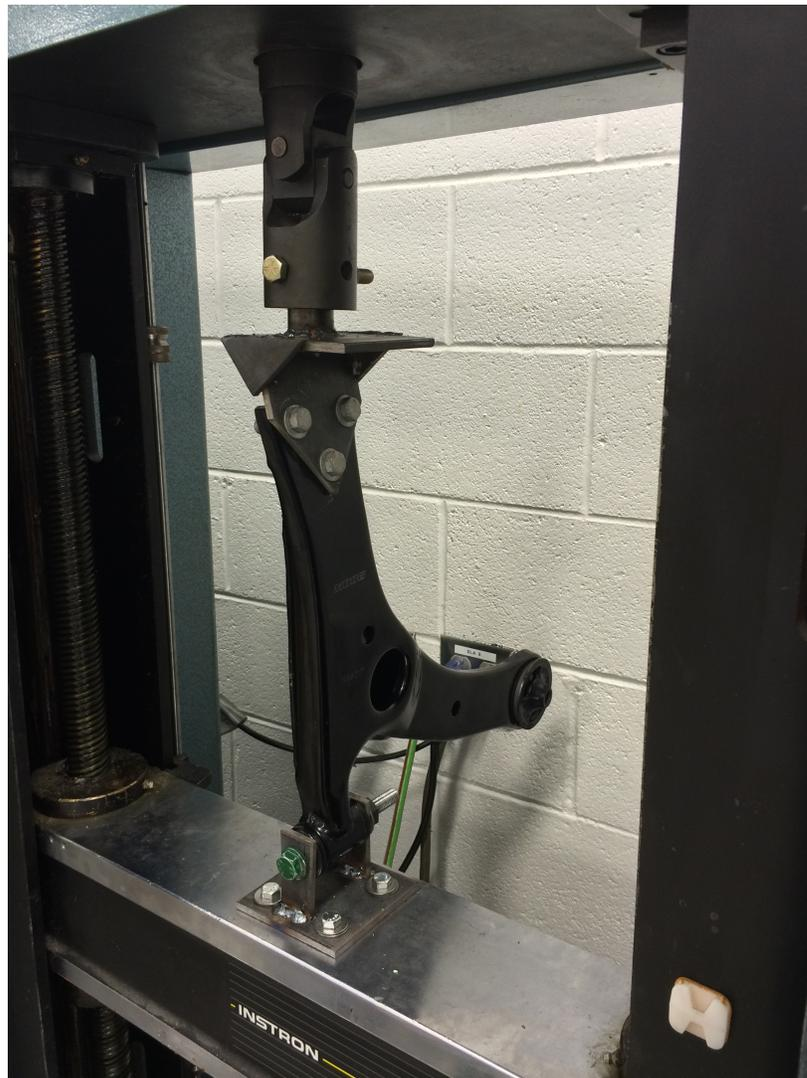
Figure 3.25: Bushing stiffness test setup.
