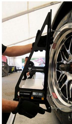
Figure 2.22: Camber measurement using camber/caster Gauge [29].
