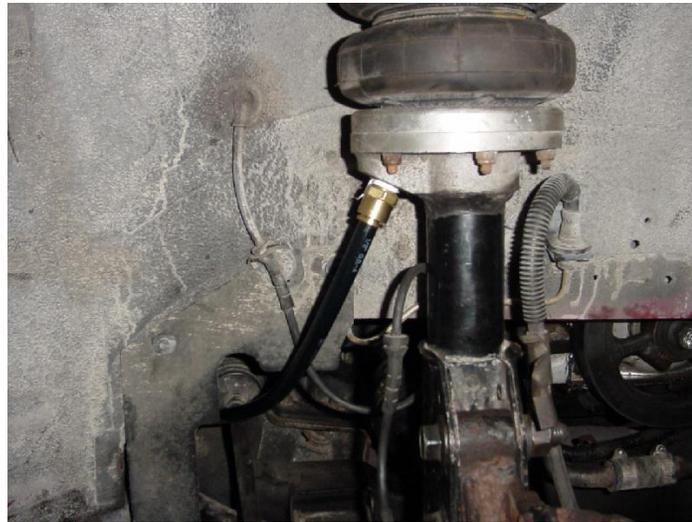
Figure 2.7: Air suspension of a Cadillac DeVille.
