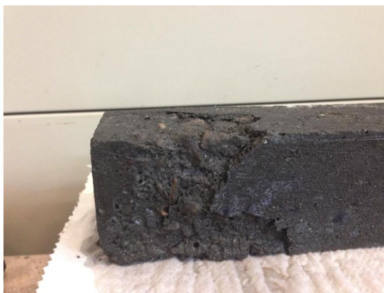
Figure: E.16 Sample 2.80.24.1 at 231 of 231 cycles.
