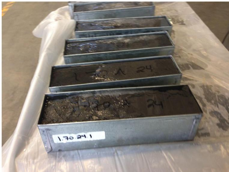
Figure: 6.7 Samples after being removed from environmental chamber.
