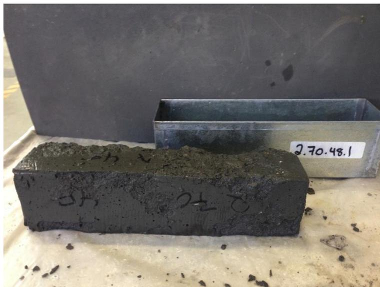
Figure: E.11 Sample 2.70.48.1 at 198 of 198 cycles.
