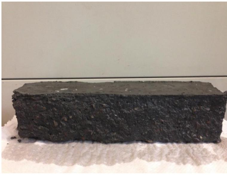
Figure: E.19 Sample 1.80.48.2 at 231 of 231 cycles.
