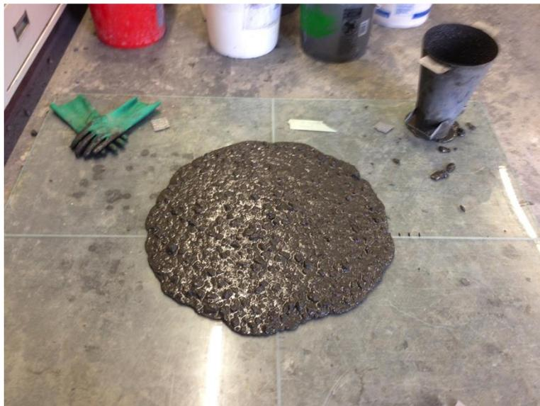
Figure: 3.2 Slump flow test sample once allowed to flow completely per ASTM C1611.
