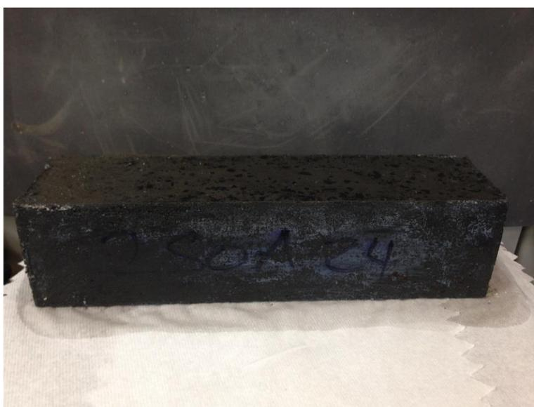
Figure: E.14 Sample 2.80.24.1 at 33 of 231 cycles.
