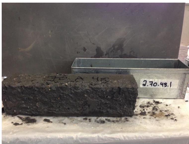
Figure: E.10 Sample 2.70.48.1 at 165 of 198 cycles.
