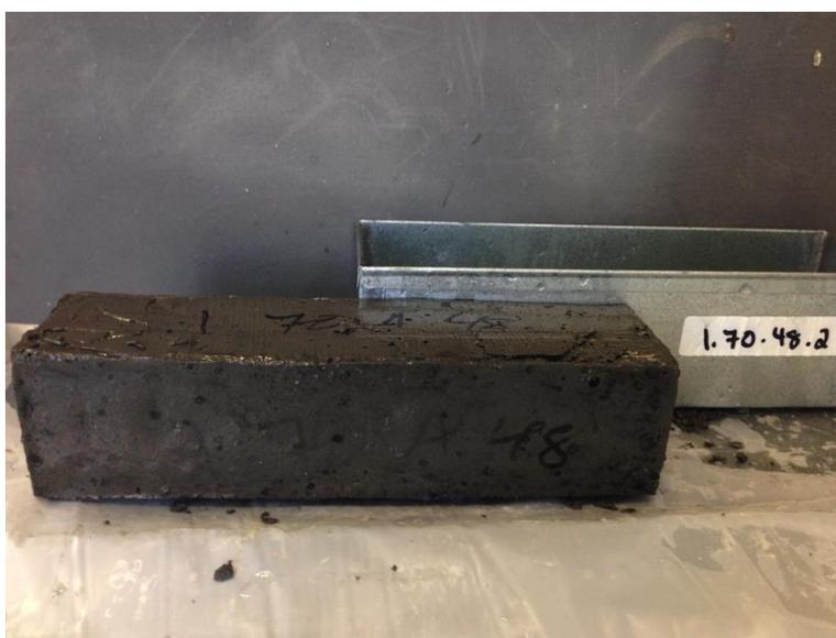
Figure: E.6 Sample 1.70.48.2 at 99 of 264 cycles.
