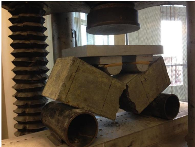
Figure: 4.14 Testing setup for modulus of rupture per ASTM C78.
