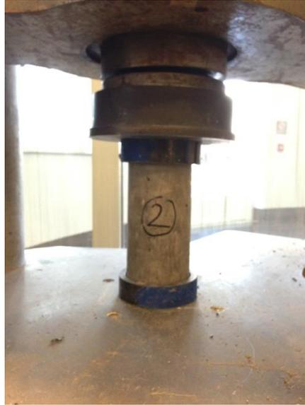
Figure: 4.4 Standard testing setup for compressive strength testing per ASTM C39.
