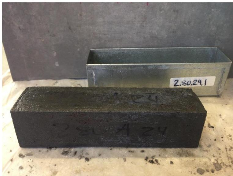
Figure: E.15 Sample 2.8.0.24.1 at 99 of 231 cycles.
