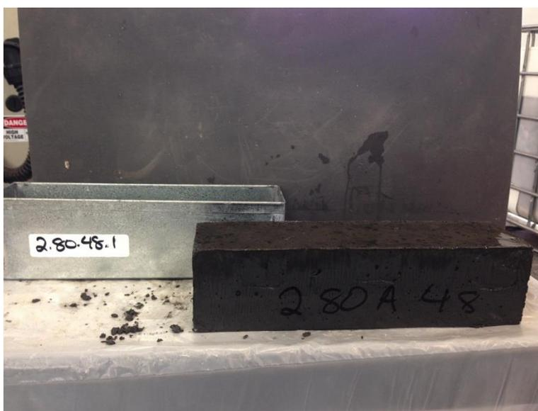
Figure: E.20 Sample 2.80.48.1 at 33 of 198 cycles.
