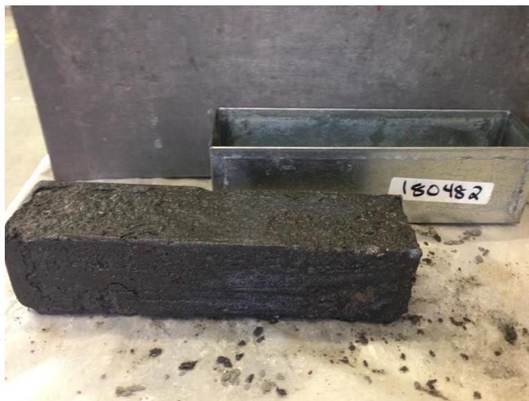
Figure: E.18 Sample 1.80.48.2 at 66 of 231 cycles.
