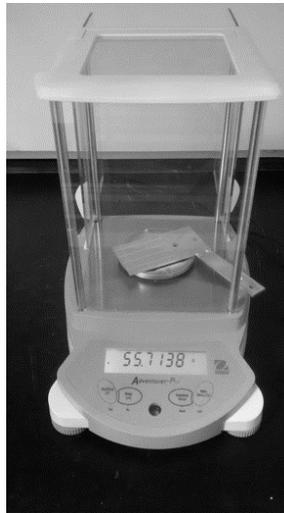
Figure 4.8 Weighing scale to measure the amount of mass loss
