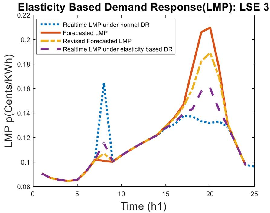
Figure 5.14: Surge mitigation (Load and LMP) under elasticity based forecasted rates (LSE 3)
