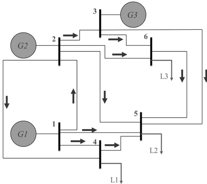
Figure 2.1: Test System: 6 Bus
