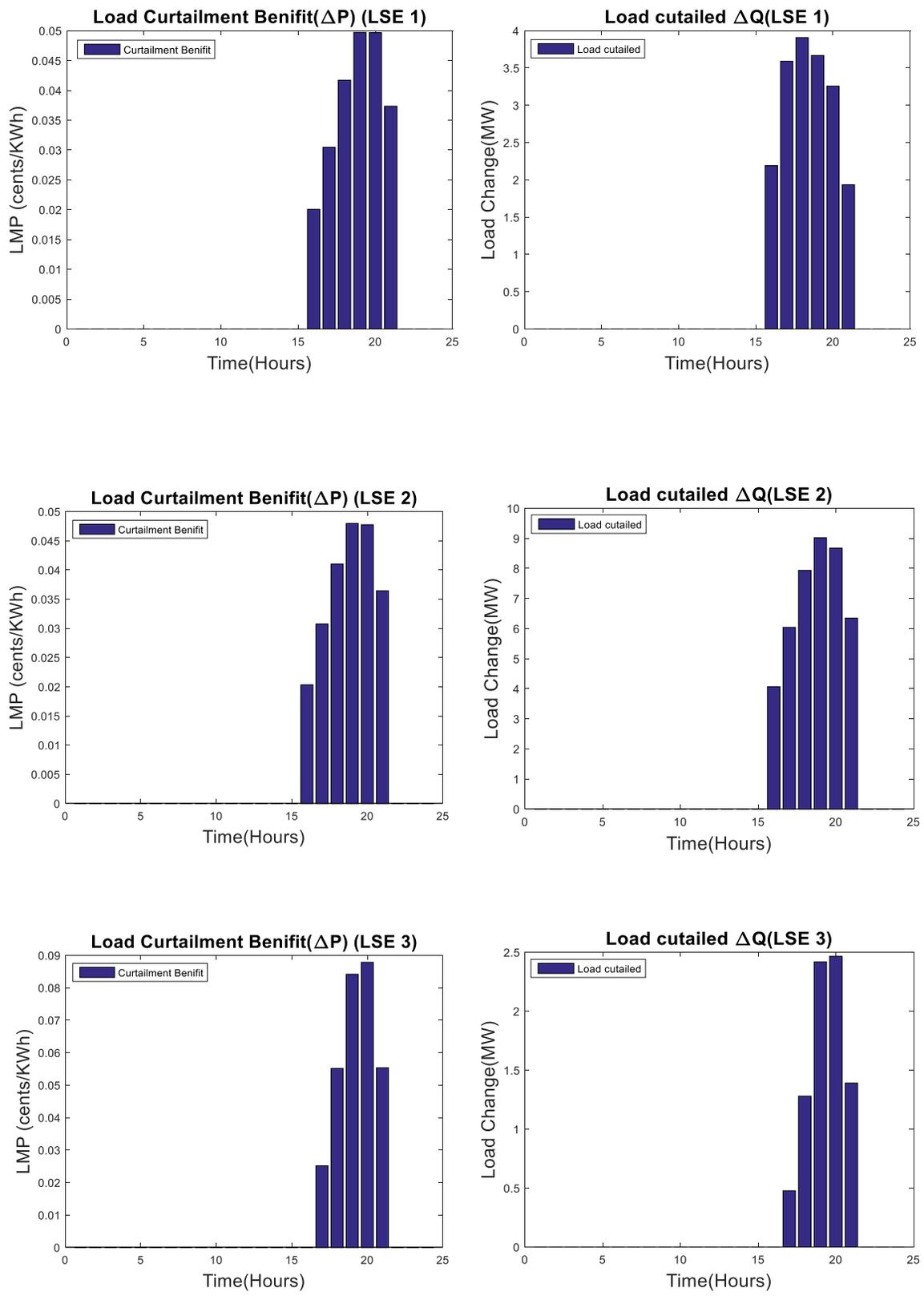
Figure 4.15: Benefit factor and corresponding load curtailment
