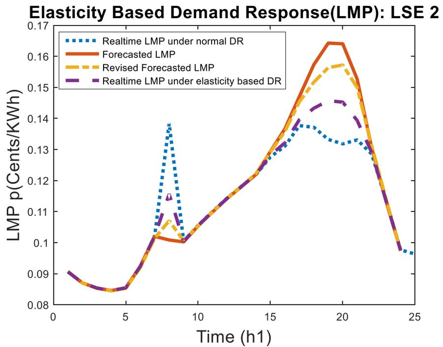
Figure 5.13: Surge mitigation (Load and LMP) under elasticity based forecasted rates (LSE 2)
