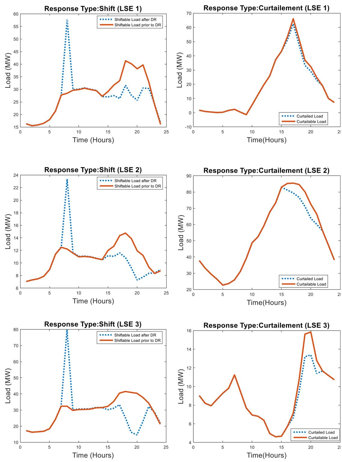
Figure 4.20: Curtailment and shift type response based on Consumer Psychology Model (Scenario 2)
