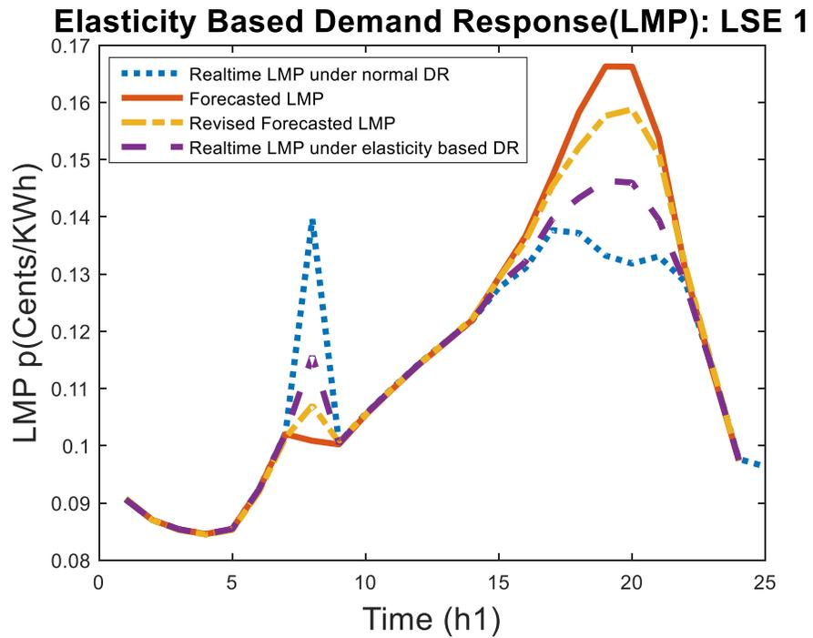
Figure 5.12: Surge mitigation (Load and LMP) under elasticity based forecasted rates (LSE 1)
