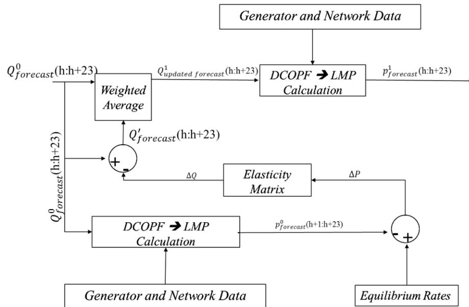
Figure 5.8: Surge mitigation using elasticity based DR
