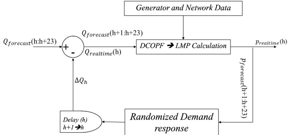
Figure 3.1: Closed loop demand response architecture
