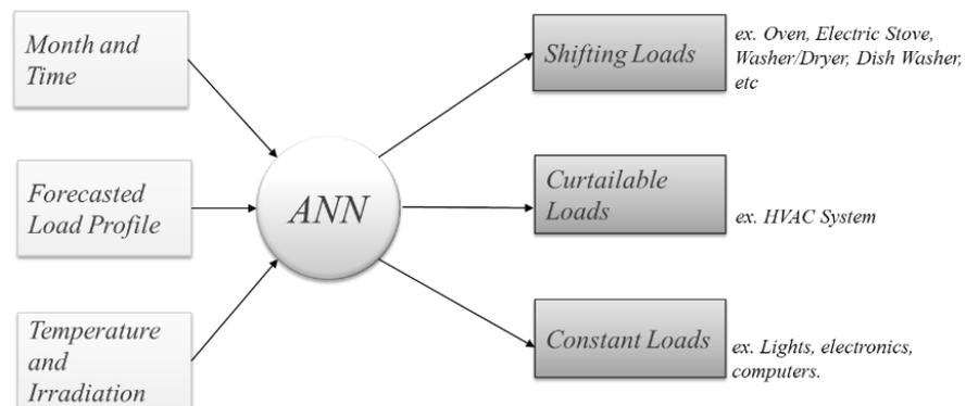
Figure 4.2: Input and output parameters of an Artificial Neural Network for load classification
