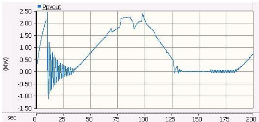
Figure 4.4 PV farm output response to changing irradiance
