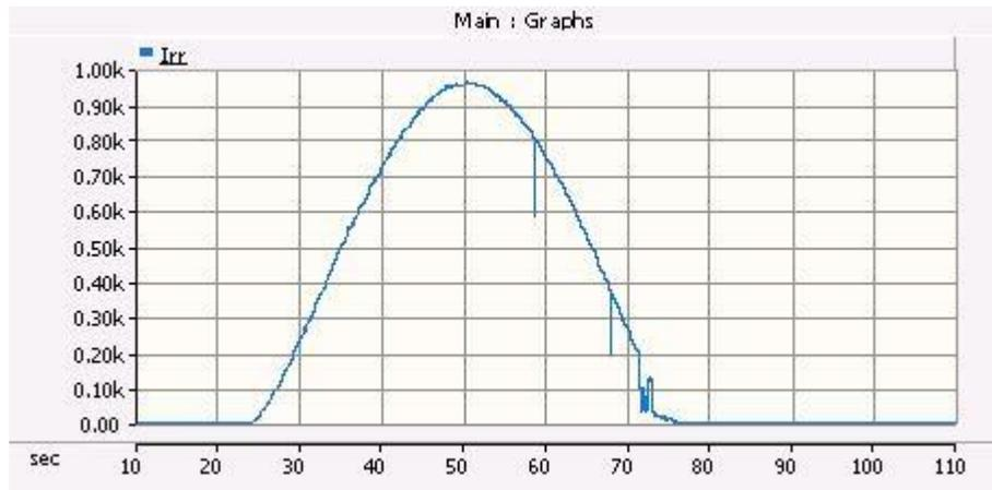
Figure 2.12 Irradiance data for a sunny day simulated between 20 seconds and 80 seconds in PSCAD
