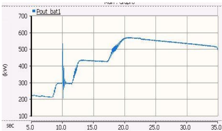
Figure 5.17 Battery response to Low frequency power demand before irradiance change
