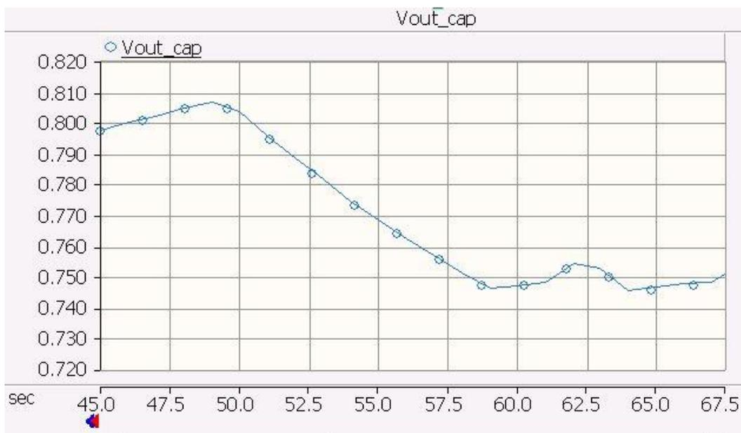
Figure 3.26 Step response in terms of voltage for UC pack [46]
