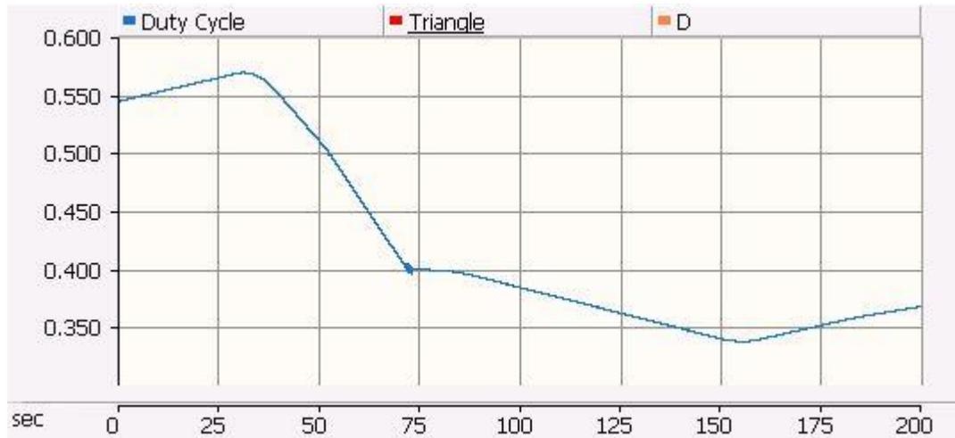
Figure 2.24 Duty ratio of the DC-DC boost converter adjusting to load demand
