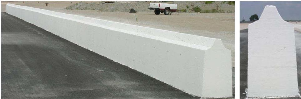
Figure 3.29: Vertical-faced concrete barrier used in the MwRSF full-scale crash test
