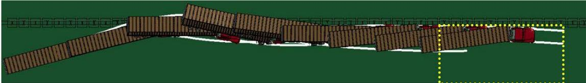
b. Case *j*: flat median wood-blockout Thrie-beam guardrail front-side impact
