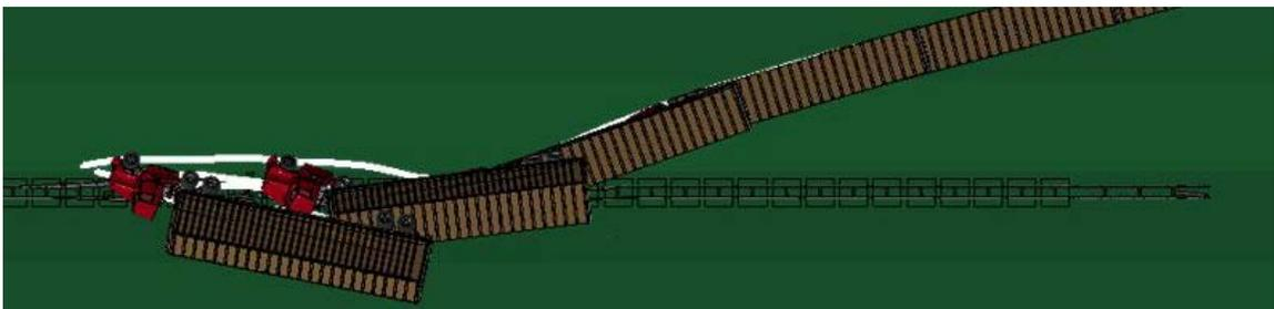
e. Case *m*: sloped median W-beam guardrail backside impact
