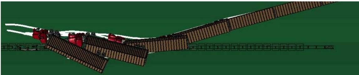
g. Case *o*: sloped median wood-blockout Thrie-beam guardrail backside impact
