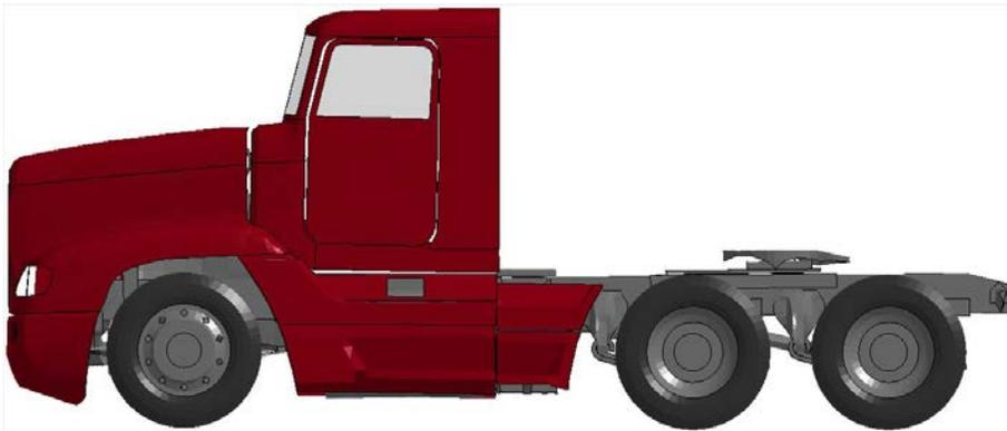
b. 154.7-in (3.9-m) wheelbase ISOL tractor FE model
