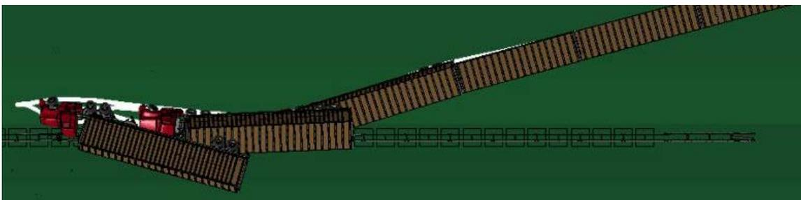
i. Case *q*: sloped median steel-blockout Thrie-beam guardrail backside impact
