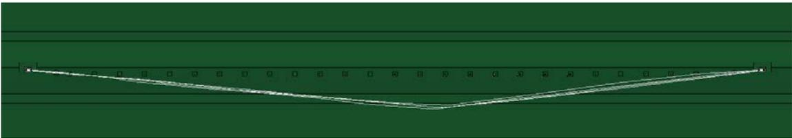
Figure A.8: Case *h*: maximum dynamic deflection, 22.4 ft (6.8 m), for the sloped median four-CMB backside impact
