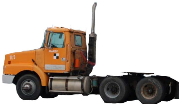
Figure 3.16: 1991 White/GMC WG64T conventional day-cab tractor used in the MwRSF full-scale crash test
