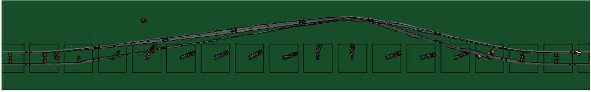
Figure A.9: Case *i*: maximum dynamic deflection, 8.6 ft (2.6 m), for the flat median W-beam guardrail front-side impact
