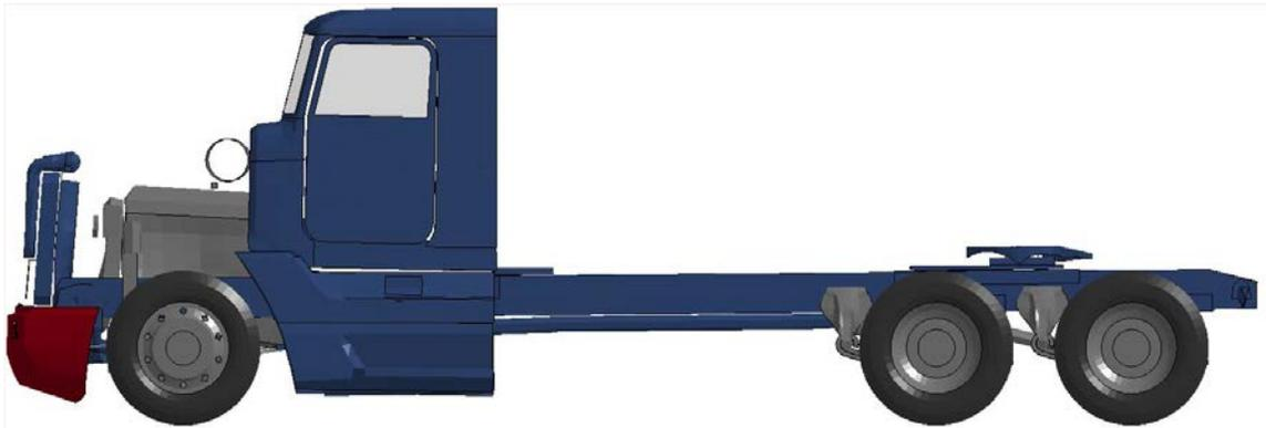
a. 217-in (5.5-m) wheelbase ISOL tractor FE model
