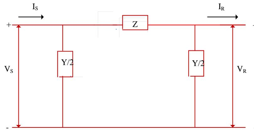
FIGURE 2.2 : Lumped type- nominal transmission( $\pi$ ) line model with  $V_S, V_R, I_S, I_R, Z, Y/2$  being sending, receiving end voltage, sending end current, receiving end current, impedance, admittance respectively [15]
