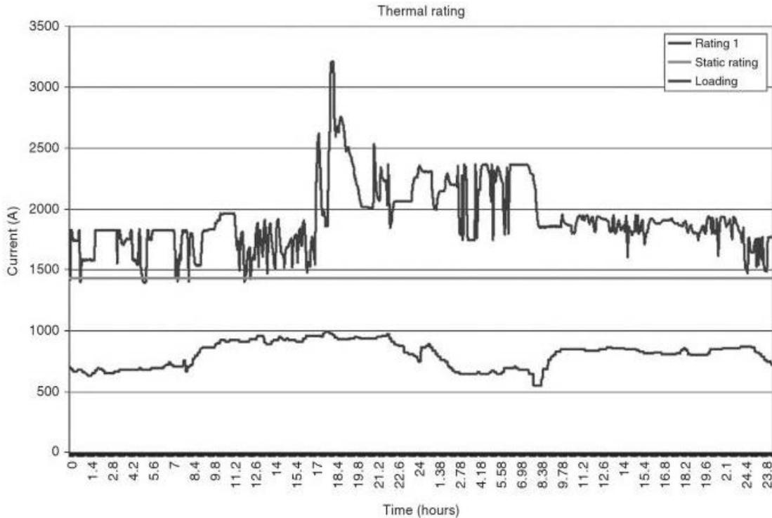
FIGURE 1.1: Dynamic thermal rating profile of a transmission line in Malaysia [14]
