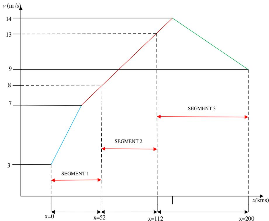
FIGURE 5.10: Wind profile  $v$  in (m/s)  $v/s$  Position ( $x$ ) in kms plotted based on wind speed measurements measured along length of transmission line in Alaska.
