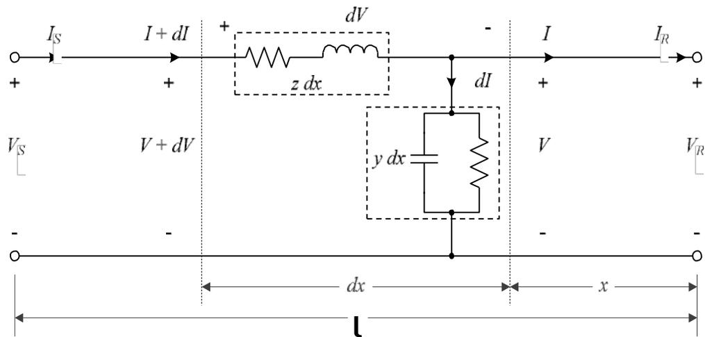
FIGURE 2.1: Uniform distributed parameter line model [22]
