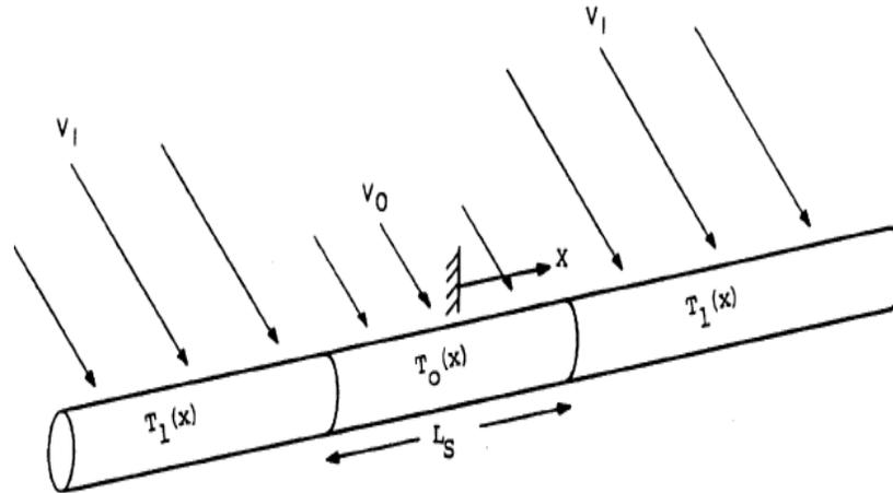
FIGURE 2.4: Wind shielding as source of non-uniformity [27]
