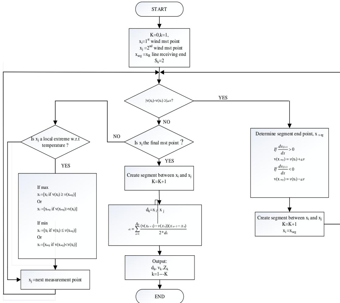
FIGURE 4.4: Flow chart representation showing algorithm for performing line model segmentation based on wind speed measurements
