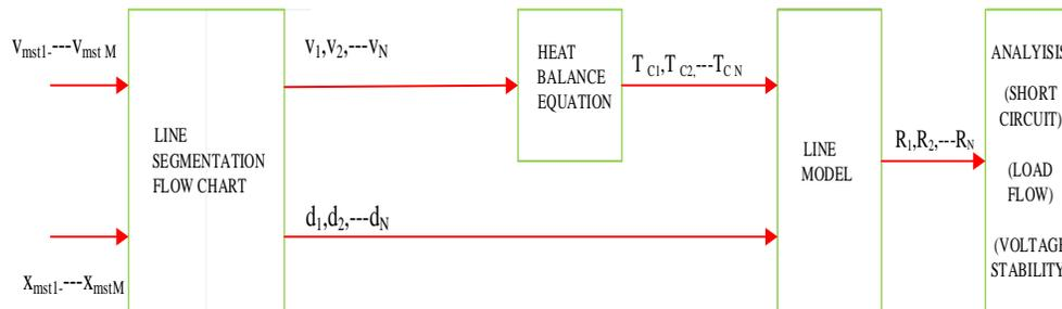
FIGURE 4.6: Proposed modeling approach with wind speed measurement inputs: measurement value ( $v_{mst1}, v_{mst2}, \dots, v_{mstM}$ ) and measurement location ( $x_{mst1}, x_{mst2}, \dots, x_{mstM}$ ), resulting line model segmentation: segment lengths and conductor temperatures ( $d_1, d_2, \dots, d_N, T_{C1}, T_{C2}, \dots, T_{CN}$ ), and resulting resistance of each segment ( $R_1, R_2, \dots, R_N$ ).
