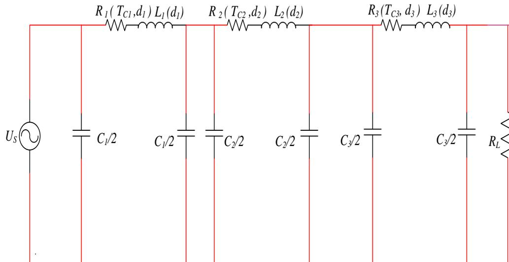
FIGURE 4.10: 3-segment line model with each line segment modeled at wind speeds ( $v_{C1}$ ,  $v_{C2}$ ,  $v_{C3}$ ) and corresponding resistances calculated at conductor temperatures  $R_1(T_{C1}, d_1)$ ,  $R_2(T_{C2}, d_2)$ ,  $R_3(T_{C3}, d_3)$ , inductances ( $L_1(d_1)$ ,  $L_2(d_2)$ ,  $L_3(d_3)$ ), capacitances ( $C_1/2$ ,  $C_2/2$ ,  $C_3/2$ ), sending-end voltage ( $U_s$ ) and resistive load ( $R_L$ ).
