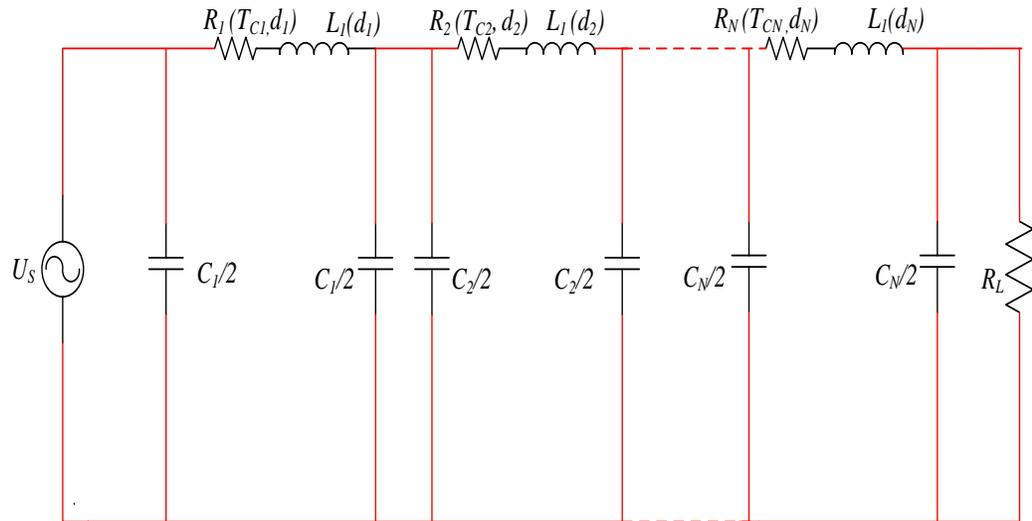
FIGURE 4.3:  $N$ -segment line model with each line segment modeled at a specific wind speed ( $v_{C1}, v_{C2}, \dots, v_{CN}$ ), each segment resistance is dependent on corresponding conductor temperature ( $R(T_{C1}), R(T_{C2}), \dots, R(T_{CN})$ ), inductance ( $L_1(d_1), L_2(d_2), \dots, L_N(d_N)$ ) and capacitance ( $C_{1/2}, C_{2/2}, \dots, C_{N/2}$ ) are independent of wind speed but depend on segment length, the load resistance is indicated by  $R_L$ .
