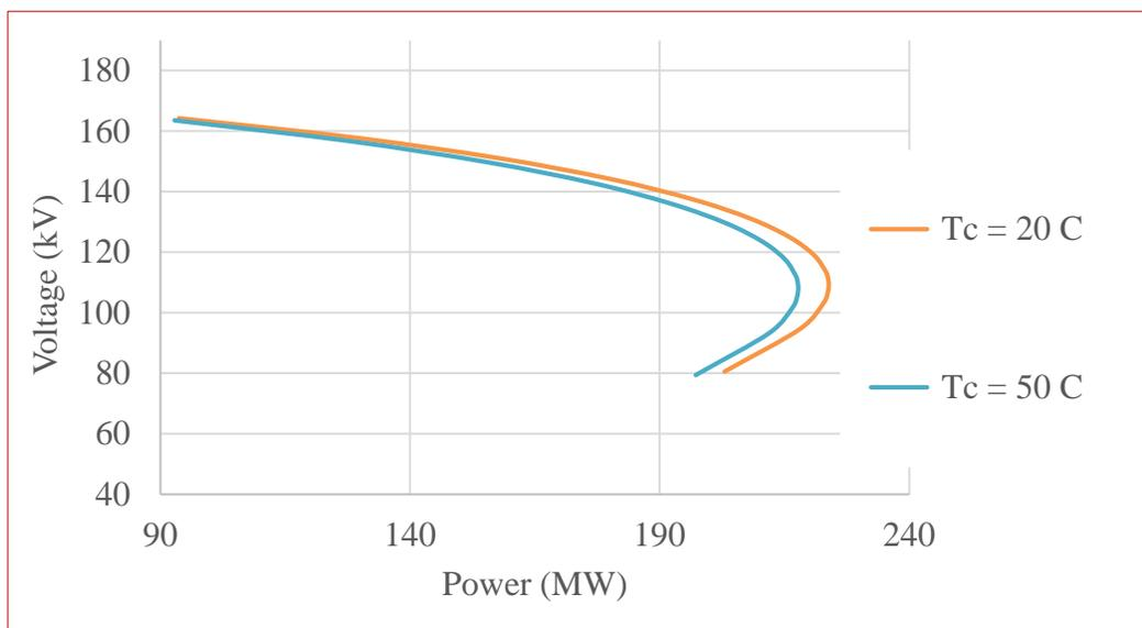
FIGURE 5.1: PV (voltage (kV) v/s power (MW)) curves for two conductor temperatures ( $T_c=20$  and  $50^\circ\text{C}$ )
