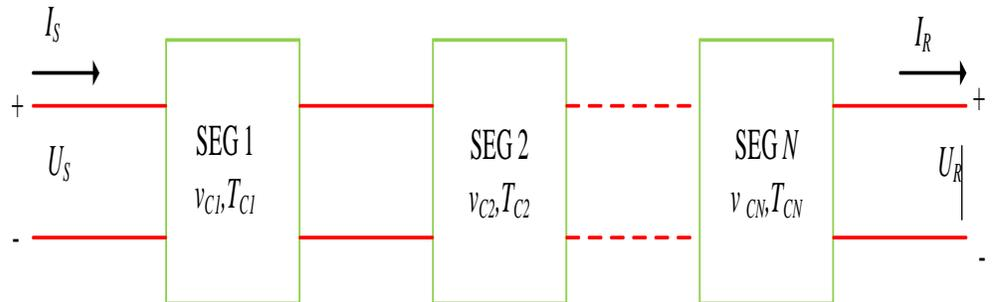
FIGURE 4.1: Block diagram of  $N$ -segment line model with each line segment at a corresponding wind speed ( $v_{C1}, v_{C2} \dots v_{CN}$ ) in m/s and corresponding conductor temperatures ( $T_{C1}, T_{C2} \dots T_{CN}$ ) in degrees Celsius ( $^{\circ}\text{C}$ ) and  $I_S, I_R, U_S, U_R$  being sending end current, receiving end current, sending end voltage and receiving end voltage respectively
