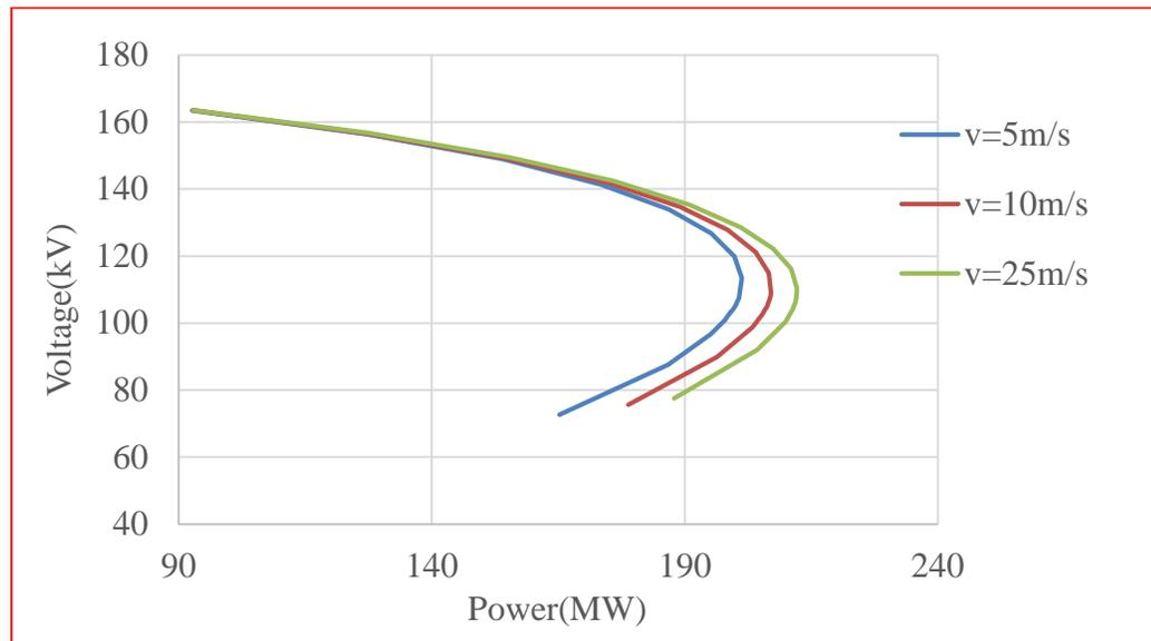
FIGURE 5.5: PV (voltage (kV) v/s power (MW)) curves for different wind speeds ( $v=5, 10, 25\text{m/s}$ )
