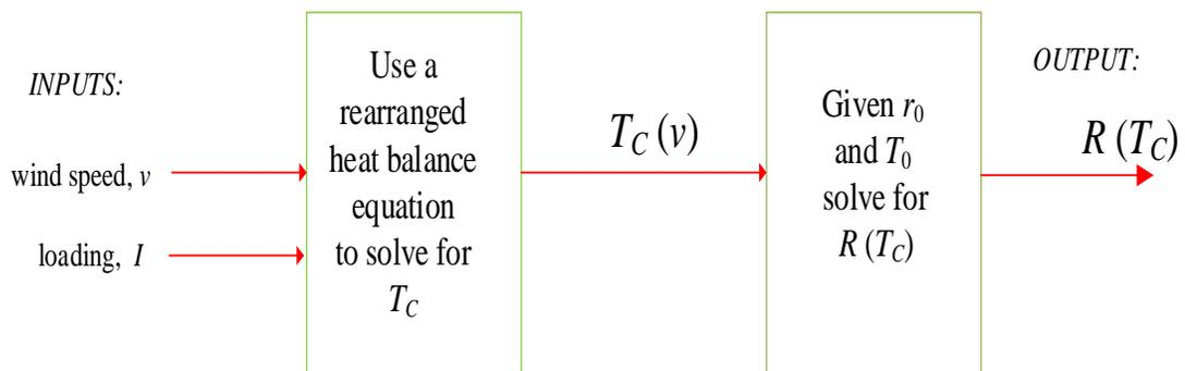
FIGURE 4.2: Proposed modeling approach with inputs (wind speed ( $v$ ) in m/s, current ( $I$ ) from steady state equation and ( $R_0$ ) being reference resistance, ( $T_0$ ) being reference conductor temperature, with conductor temperature ( $T_C$ ), line resistance of conductor  $R(T_C)$ ) and outputs (power in (MW) and receiving end voltage ( $U_R$ )),  $d$  is the length of the line
