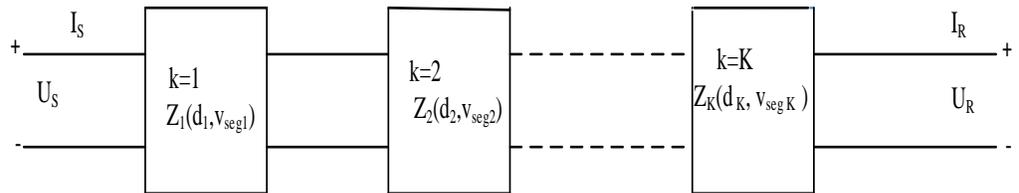
FIGURE 3.2: Representation of model structure for cascaded network of  $K$ -Segments, each at different wind Speed (and subsequently different  $T_c$ ) [19]
