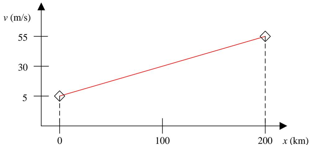
FIGURE 5.6: Graphical representation of example wind profile and two possible ways to incorporate wind speed information within the line model.
