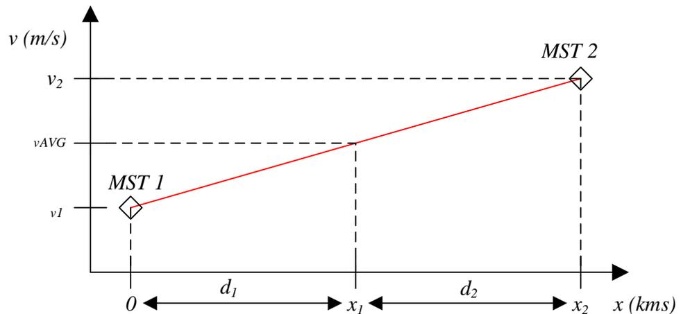
FIGURE 4.7: Representation of wind profile  $v$  dependent on distance  $x$
