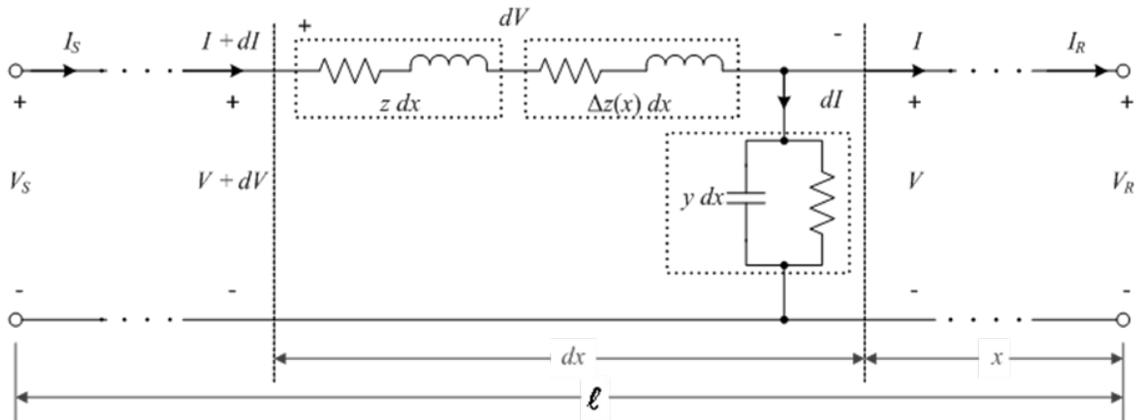
FIGURE 3.1: Non-uniform distributed line model [20]
