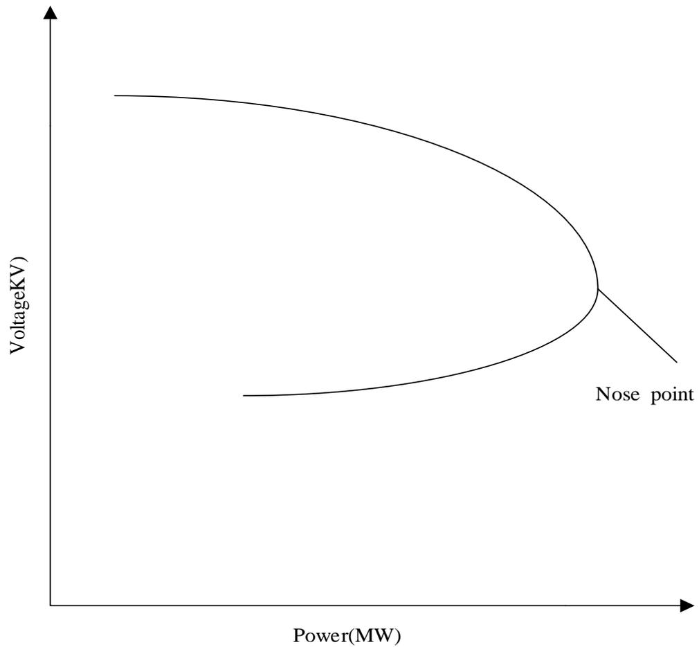
FIGURE 4.11: A simple PV curve with its nose point [29]
