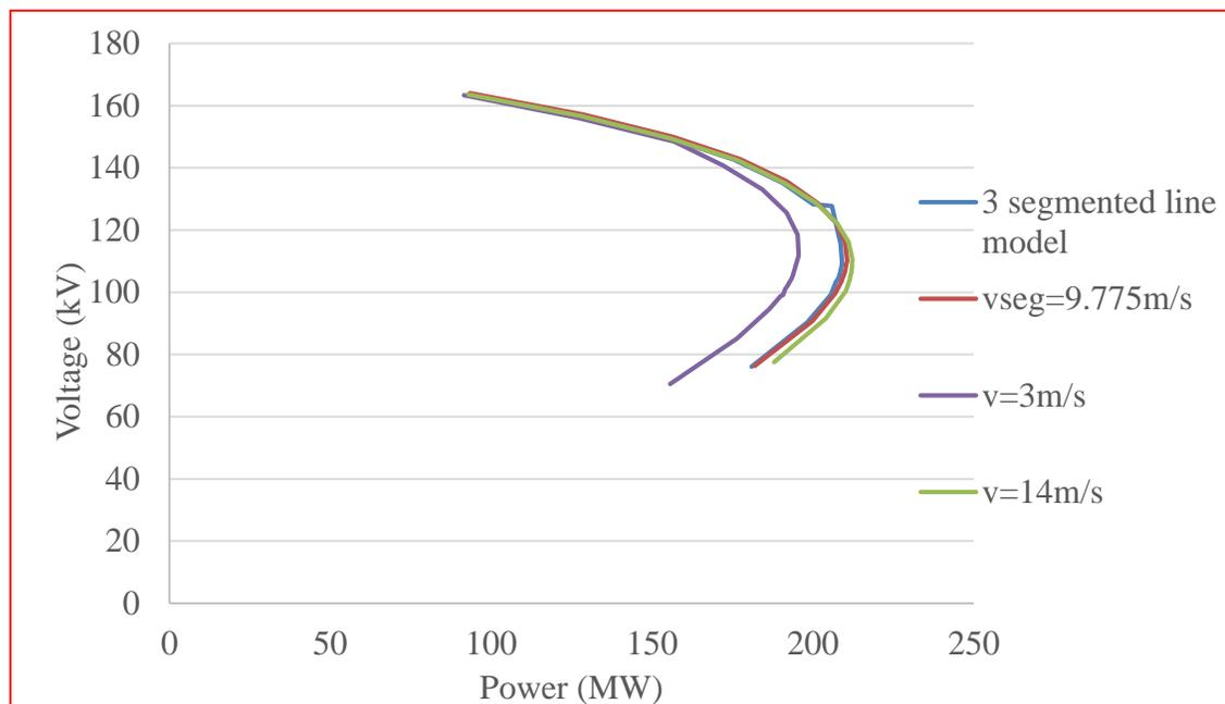
FIGURE 5.12: Voltage stability curves (voltage (kV) v/s power (MW)) graph drawn for line divided into 3-non-uniform segments, highest and lowest wind measurements and wind speed at weighted average
