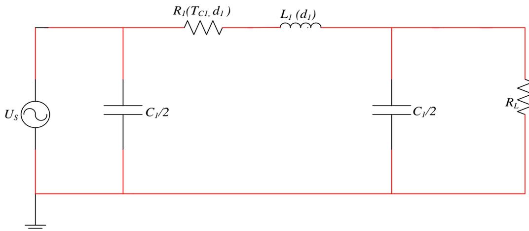
FIGURE 4.5: ( $\pi$ ) Line model with single line segment having sending end voltage ( $U_s$ ), resistance of line dependent on conductor temperature ( $T_{C1}$ ), with inductance ( $L_l$ ), capacitance divided in two halves ( $C_1/2$ ), ( $C_1/2$ ), load resistance ( $R_L$ ).
