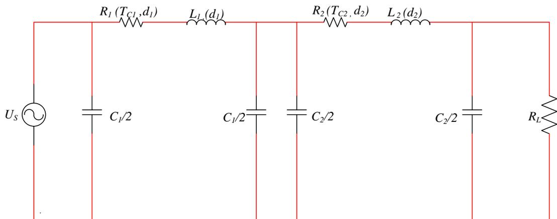
FIGURE 4.8: 2-segment line model with each line segment modeled at wind speed ( $v_{avg1}$  and  $v_{avg2}$ ) respectively, resistances calculated at corresponding conductor temperatures  $R(T_{C1})$  and  $R(T_{C2})$ , inductances ( $L_1(d_1)$  and  $L_2(d_2)$ ) and capacitances ( $C_1/2$  and  $C_2/2$ ), sending-end voltage ( $U_S$ ) and load resistance ( $R_L$ ).
