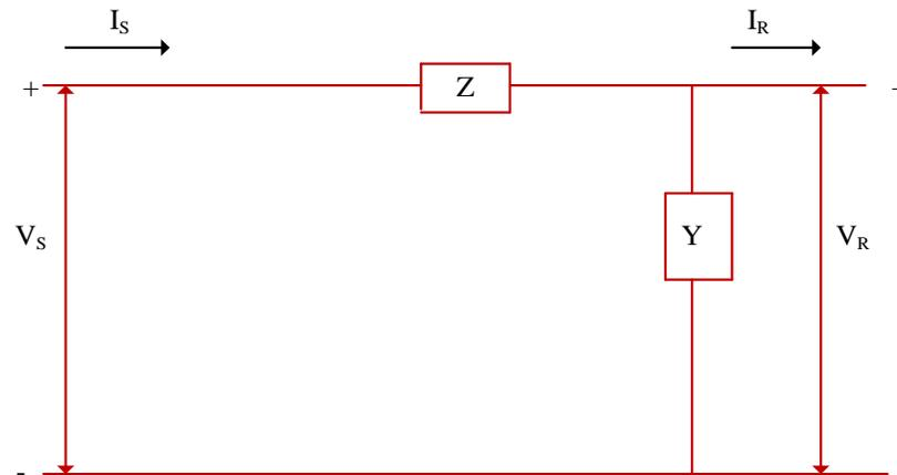
FIGURE 2.3: Lumped type- nominal transmission( $\tau$ ) line model with  $V_s, V_R, I_s, I_R, Z, Y$  being sending ,receiving end voltage, sending end current, receiving end current, impedance, admittance respectively [15]
