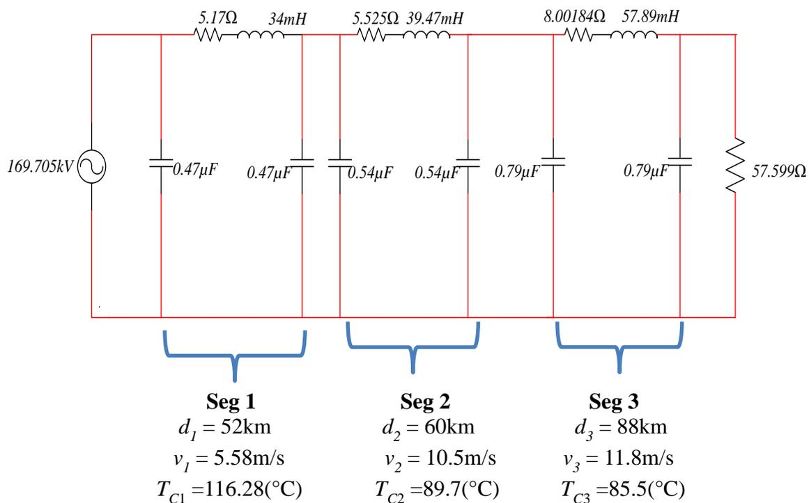
FIGURE 5.11: Representation of 3 non-uniform segmented transmission line
