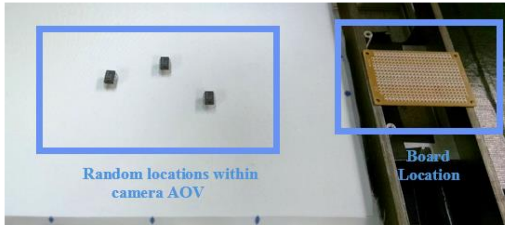
Figure 44: LM311 experimental component placement overview
