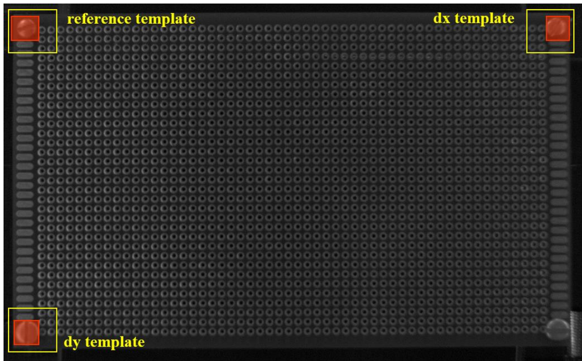
Figure 41: Board placement template overview
