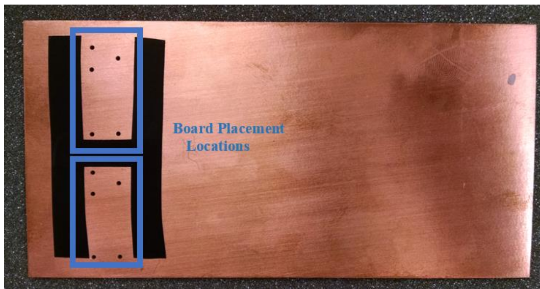
Figure 61: Custom machined circuit board for JQX-118F component
