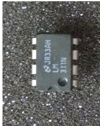
Figure 42: LM311 component (top view)
