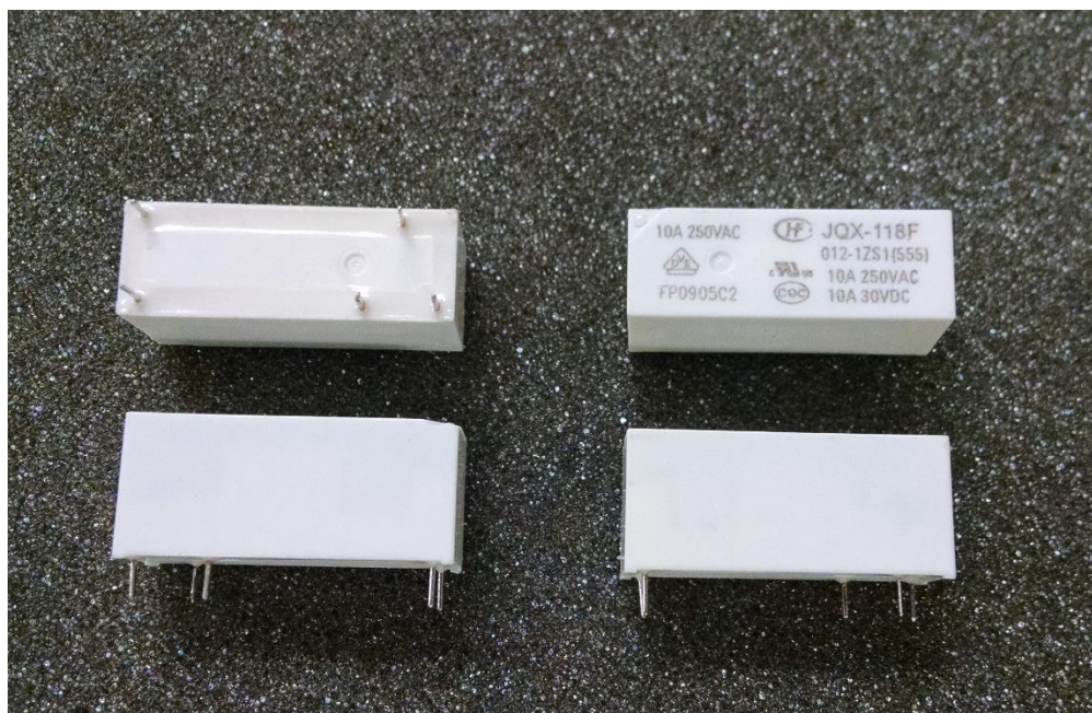
Figure 60: JQX-118F component features
