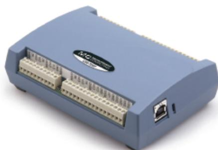
The USB-TEMP Series provides temperature measurement flexibility as each channel can monitor any of the supported input types
