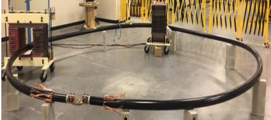
*Figure 5: Sample cable looped as secondary*
