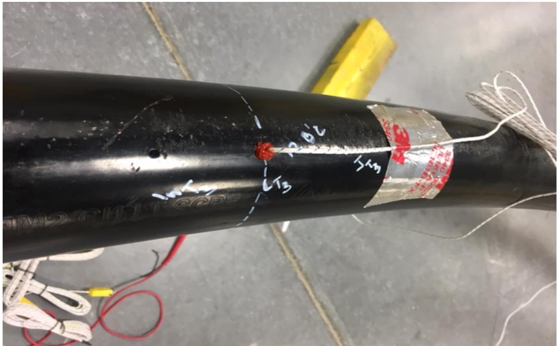
Figure 10: Conductor thermocouple installation
