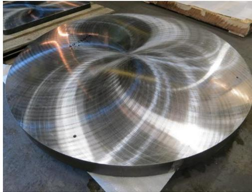
FIGURE 4.18 A Blanchard ground part showing a crosshatch pattern.
