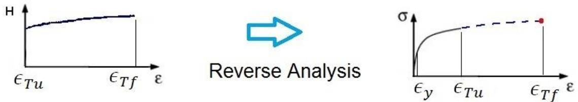
FIGURE 4.8: Schematic of the reverse analysis performed. Plastic strain ranges for measured nanohardness (left) and flow curve (right).
