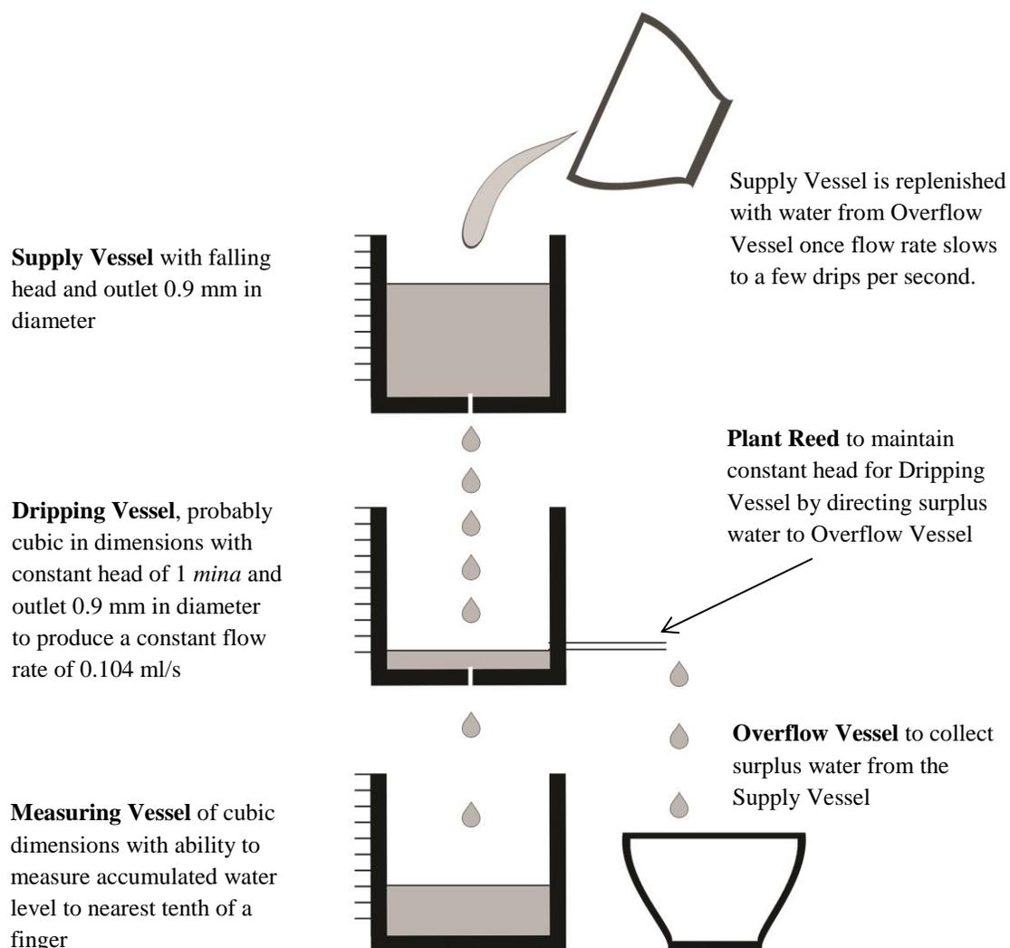
FIGURE 2: Potential design of water clock for Old Babylonian period
