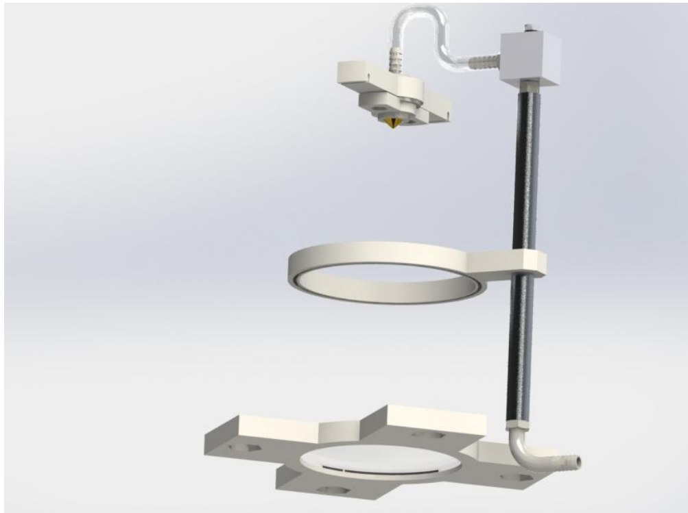
Figure 36: Base, middle, and top of spray chamber and injection unit
