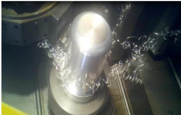
Figure 1.1: Chip nest created by a standard metal turning process. These are often dangerously sharp and can damage the part and surface finish.
