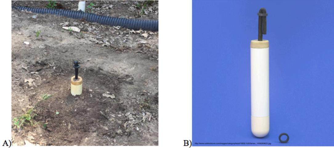
Appendix Figure 1: A) An installed lysimeter in a rain garden. B) A profile view of the 1900L Near Surface Samplers installed at each rain garden.
