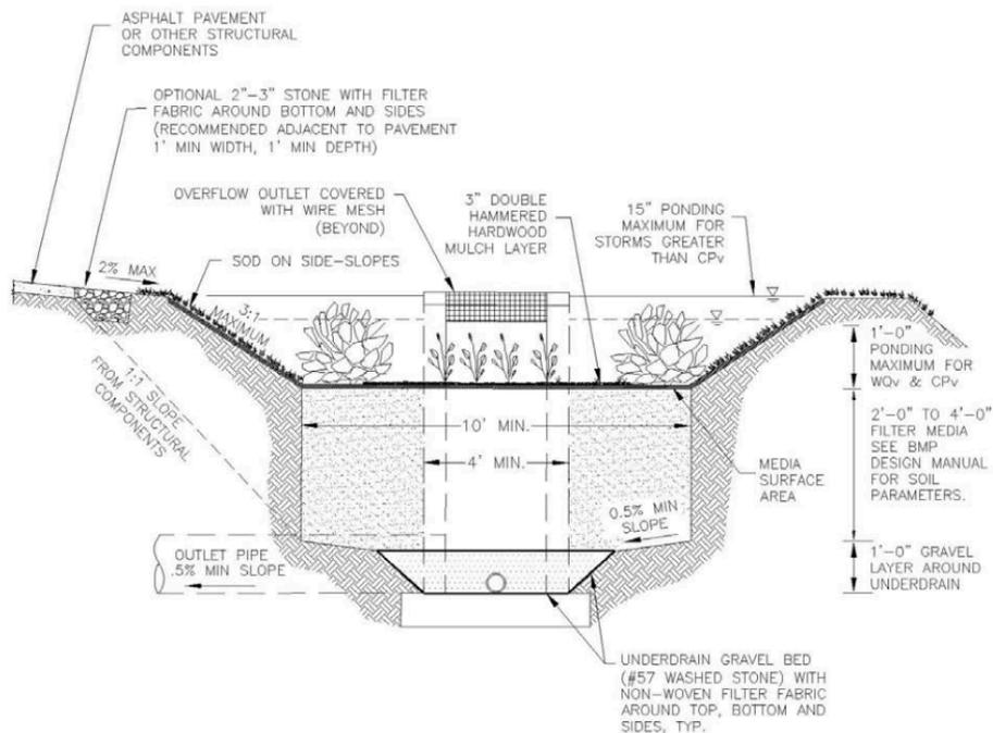
Figure 6: A cross section of a typical rain garden as diagramed in the Charlotte stormwater best management practices manual (Charlotte-Mecklenburg Storm Water Services 2014).
