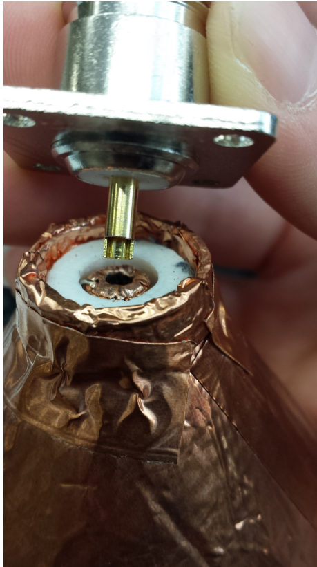
Figure A.1: Photo of connection between N-connector and 3D printed taper.
