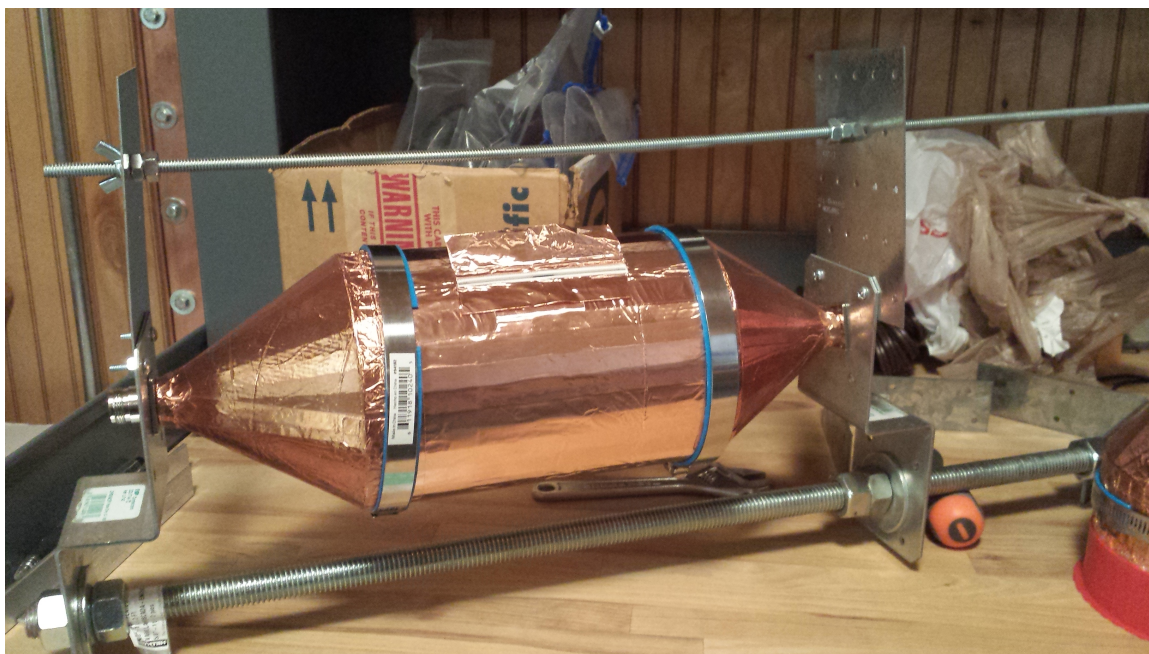
Figure A.17: Photo of the completed measurement fixture/Line standard.
