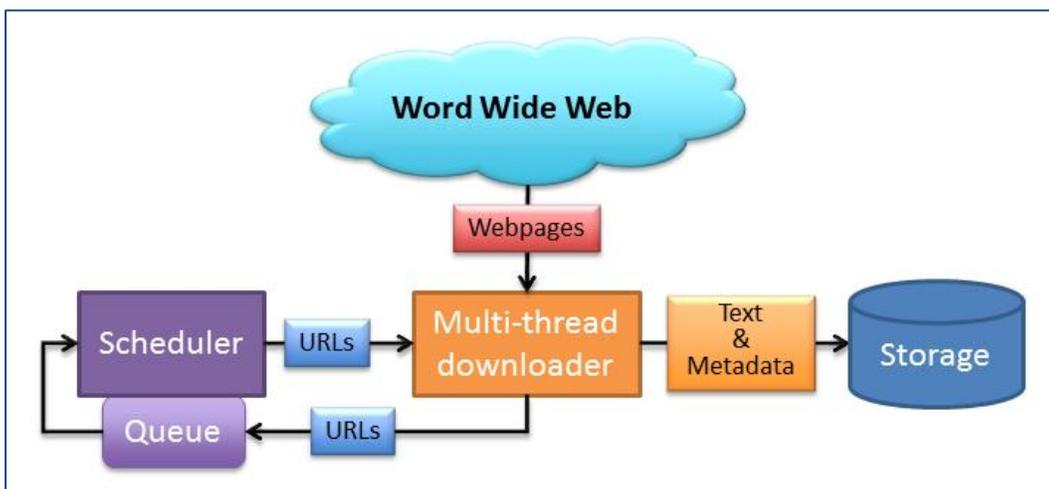
Figure 5.7: Simple architecture of the Web crawler
