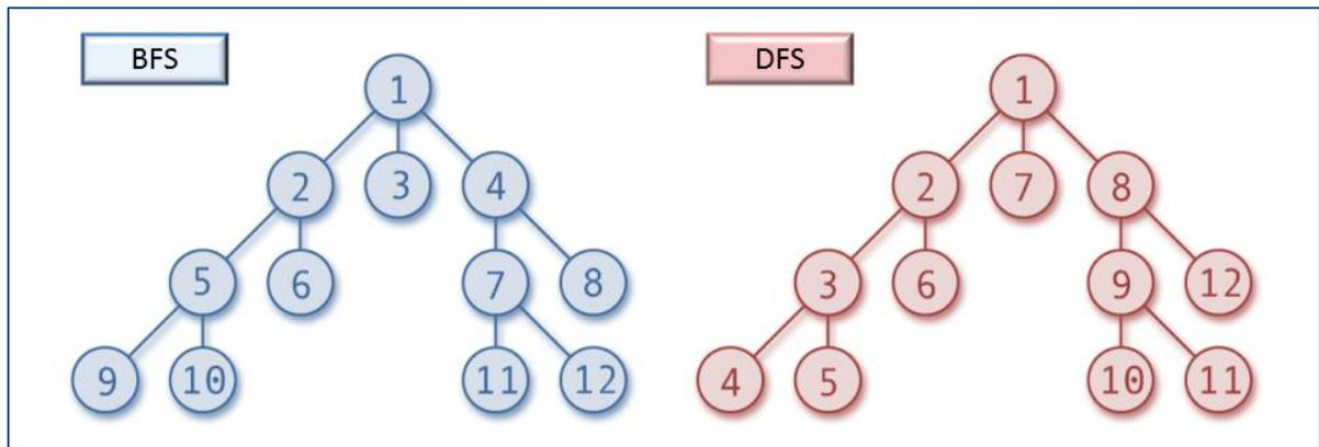
Figure 5.8: Breadth-first Search and Depth-first Search (adapted from the Wikimedia Commons file “Breadth-first-tree.png” <http://commons.wikimedia.org/wiki/File:Breadth-first-tree.png> and “Depth-first-tree.png” <http://commons.wikimedia.org/wiki/File:Depth-first-tree.png>)
