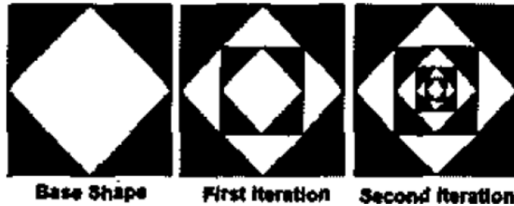
Figure 16: A “crown square fractal” patch antenna from [57].
