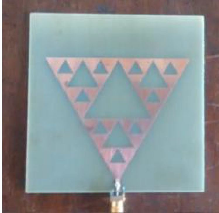
Figure 17: A multiband fractal patch antenna based on a Sierpinski gasket from [59].
