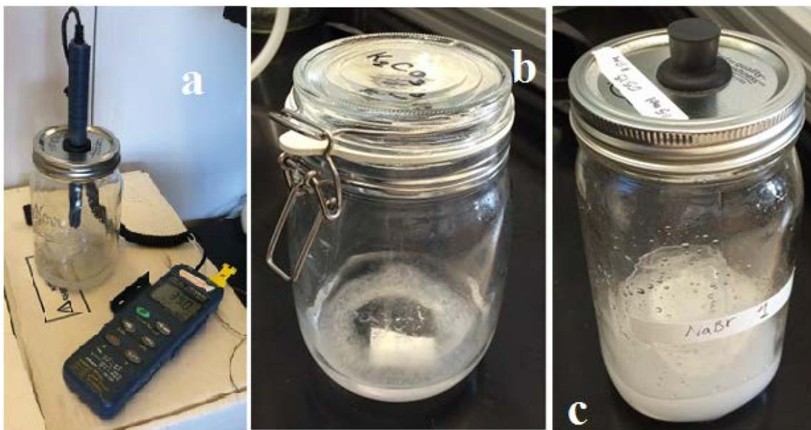
Figure 2.1: a. EOMEGA HH134A humidity meter with wired probe, b. Kilner jar, c. Mason jar
