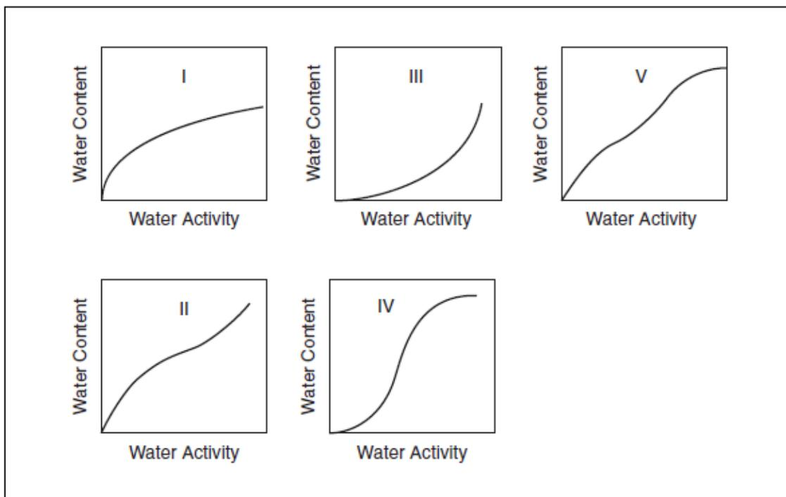
Figure 1.3: Sorption isotherm graphs presented by Brunauer *et al* [12]
