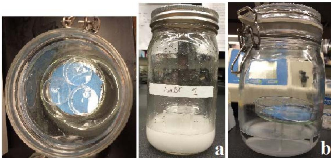
Figure 2.4: Position of samples within plastic petri dishes on pizza stand above saturated salt surface level in preserving jars, a. Mason jar, b. Kilner jar
