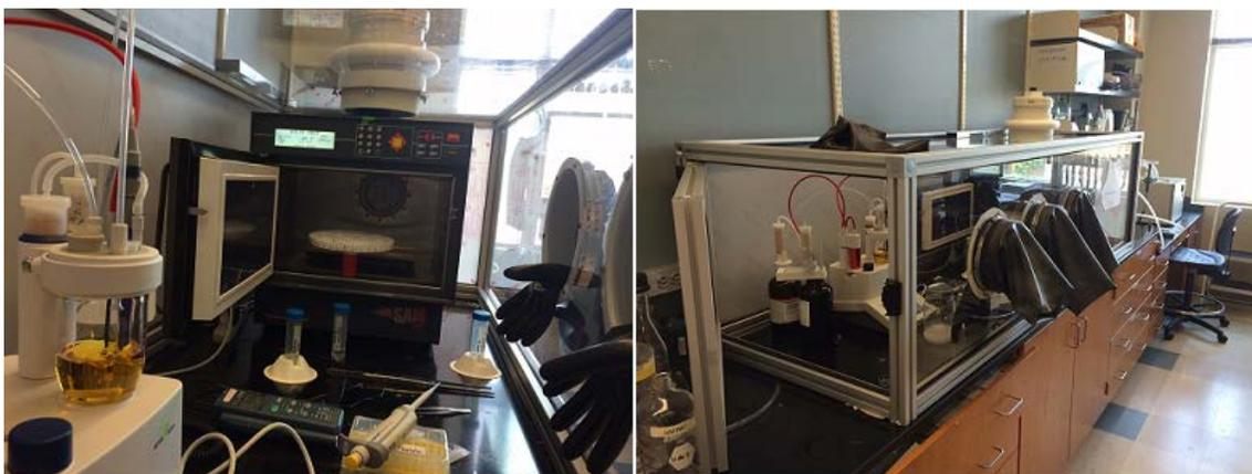
Figure 2.2: Arrangement of volumetric KF titration and microwave device inside the glove box
