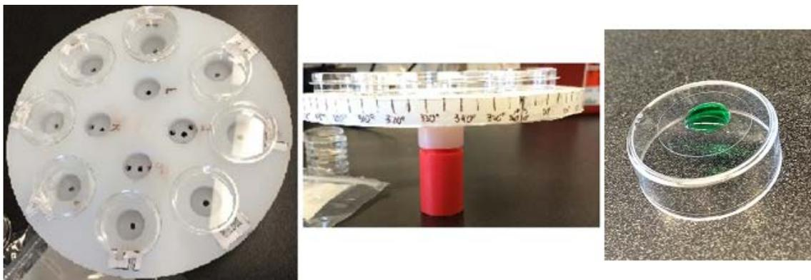
Figure 2.3: Microwave turn table with plastic petri dishes on outer ring, sample on a cover slip on top of a plastic petri dish
