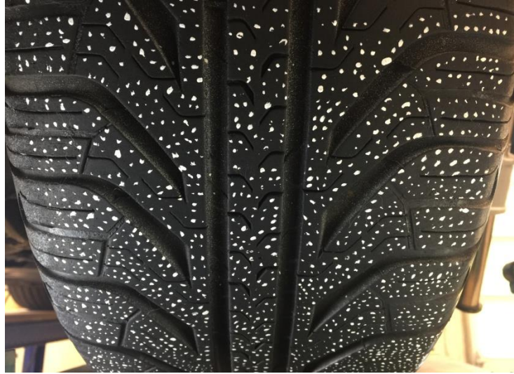
Figure30: Tire with paint for displacement measurement
