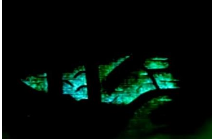
Figure 22: Tire footprint using FTIR at 2.3^{\circ} camber
