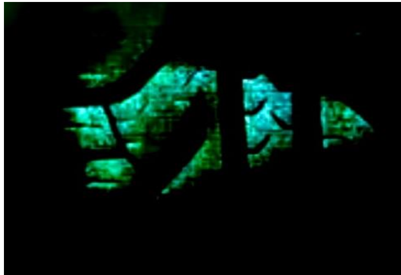
Figure 24: Initial footprint image for 2.3 0 camber
