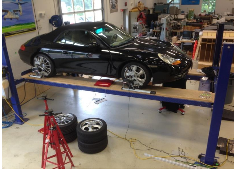
Figure 15: modified 4 post lift set up
