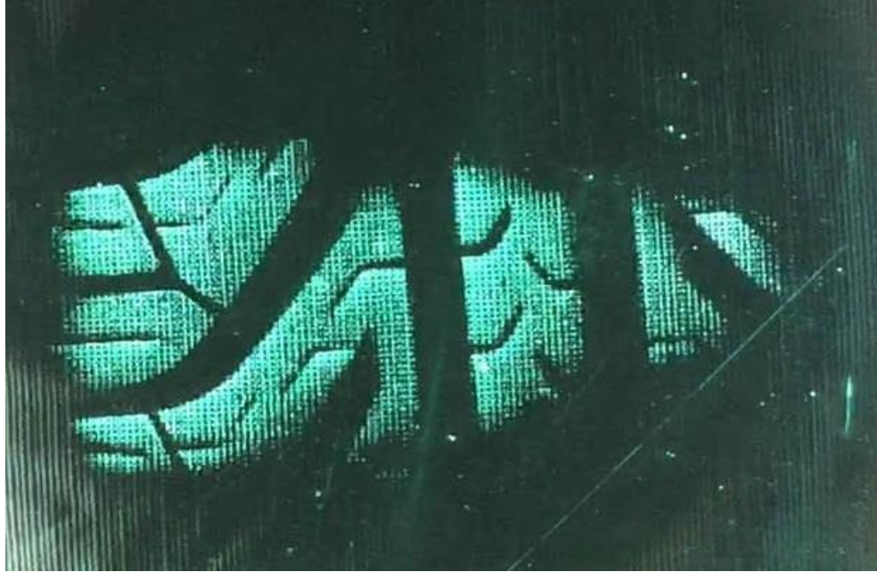
Figure 25: Footprint images for 2.3^{\circ} camber after method modification
