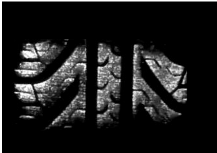
Figure 27: gray scale footprint for 0^{\circ} camber after deleting noise
