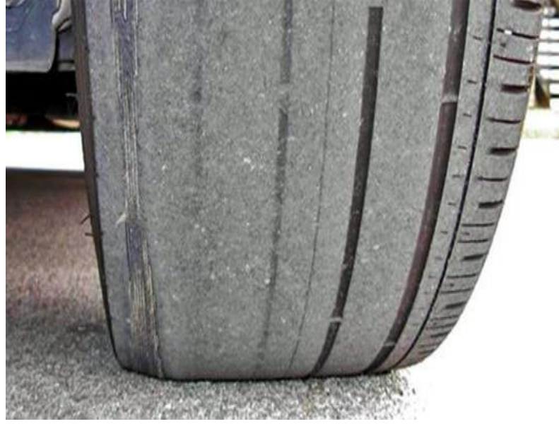
Figure 10: Tire wear due to camber [4]
