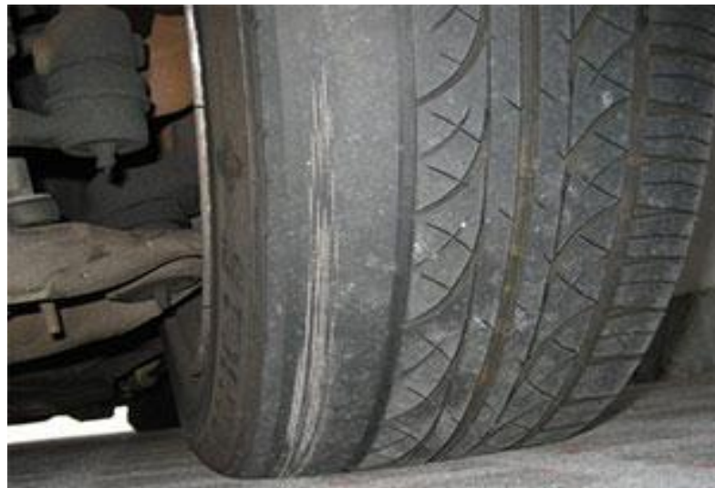
Figure 9: Shoulder wear due to camber [4]
