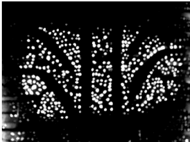
Figure 31: Tire footprint with sprayed paint at 6^{\circ} slip angle
