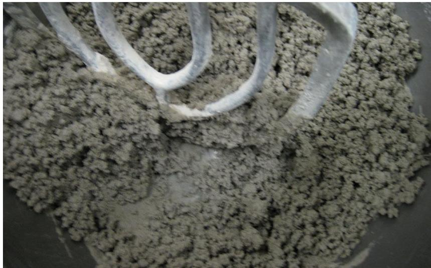
Figure 3.9: Mixed Kaolin Clay-Ottawa Sand Soil Beginning to Cohere
