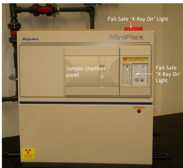
Figure 3.18: Rigaku Miniflex+ XRD
