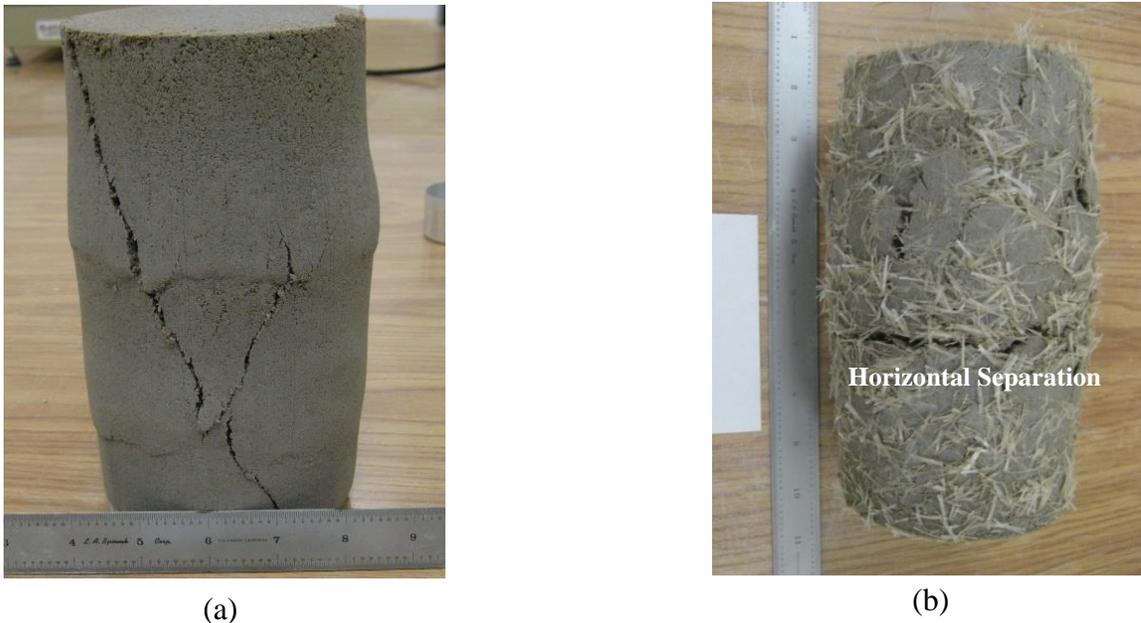
Figure 4.12: Typical Failures: (a) Angular Shear; (b) Bulging with Horizontal Separation
