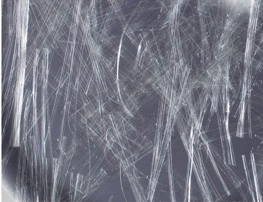
Figure 3.5: FIBERCAST 500™ Polypropylene Fibrillated Fiber
