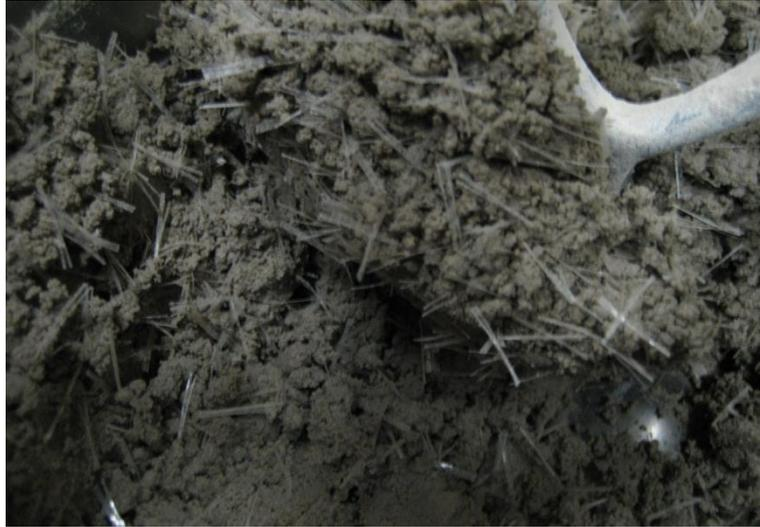
Figure 3.10: Final Soil Mix after the Addition of Fiber Reinforcement
