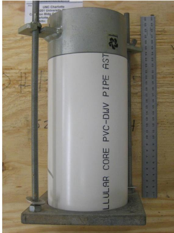
Figure 3.6: Custom Compaction Mold Used to Generate the Test Specimens
