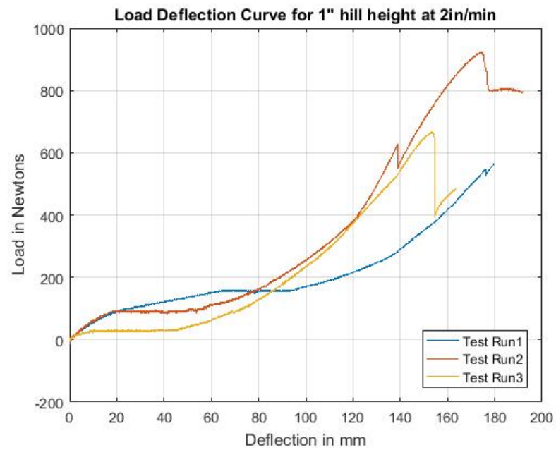
Figure 8.12: Load Deflection data of Design 1 for a strain rate of 2in./min.
