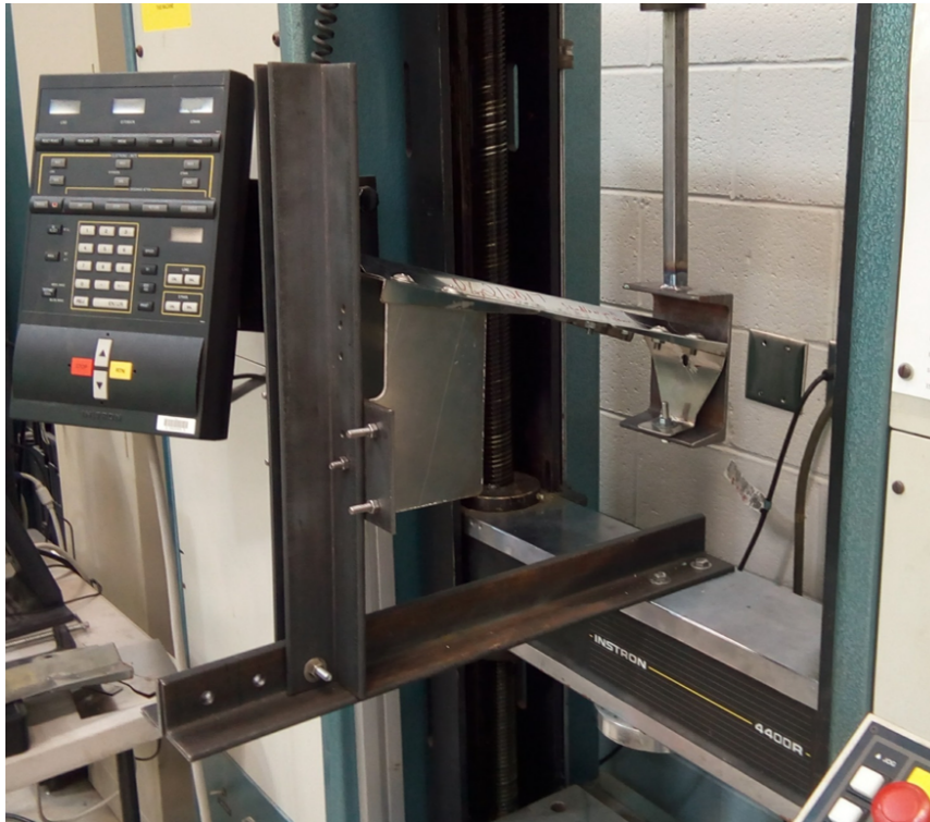
Figure 8.2: Fixture and bracket mounted on Instron test machine.
