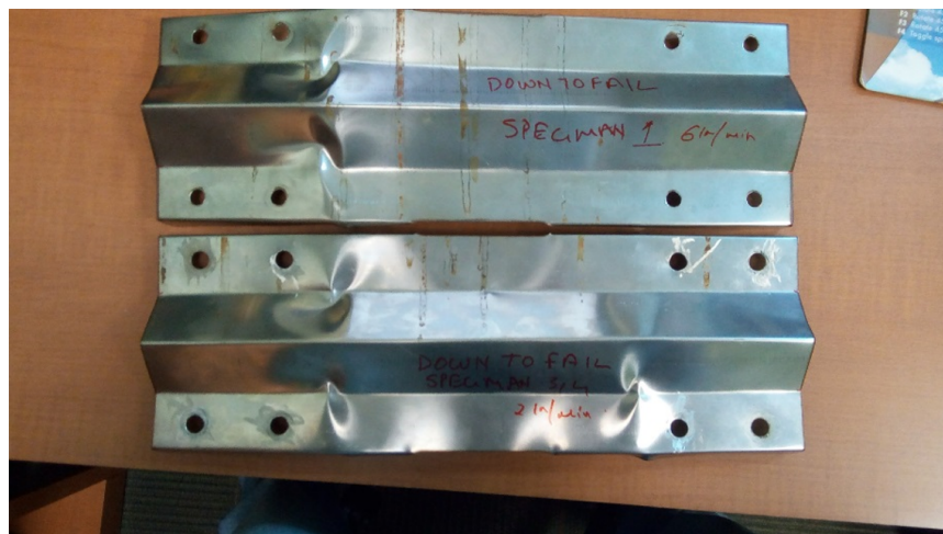
Figure 8.13: Deformed shape of the parts after the buckling test. Top sample shows loading rate at 6in./min. Bottom sample shows loading rate at 2 in./min.
