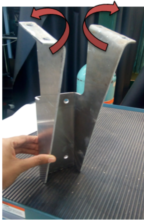
Figure 6.8: Bracket Rear for preliminary design, highlighting deflection.
