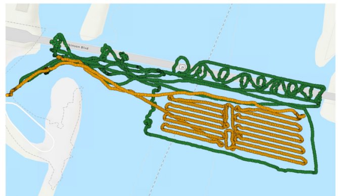
Fig. 4. Two data collection runs were executed using the HyDrone uncrewed surface vessel. The first run (green markers) consisted of a remotely piloted survey in the vicinity of the bridge and an outline of a "box" in which to conduct the second automated survey (orange markers).
