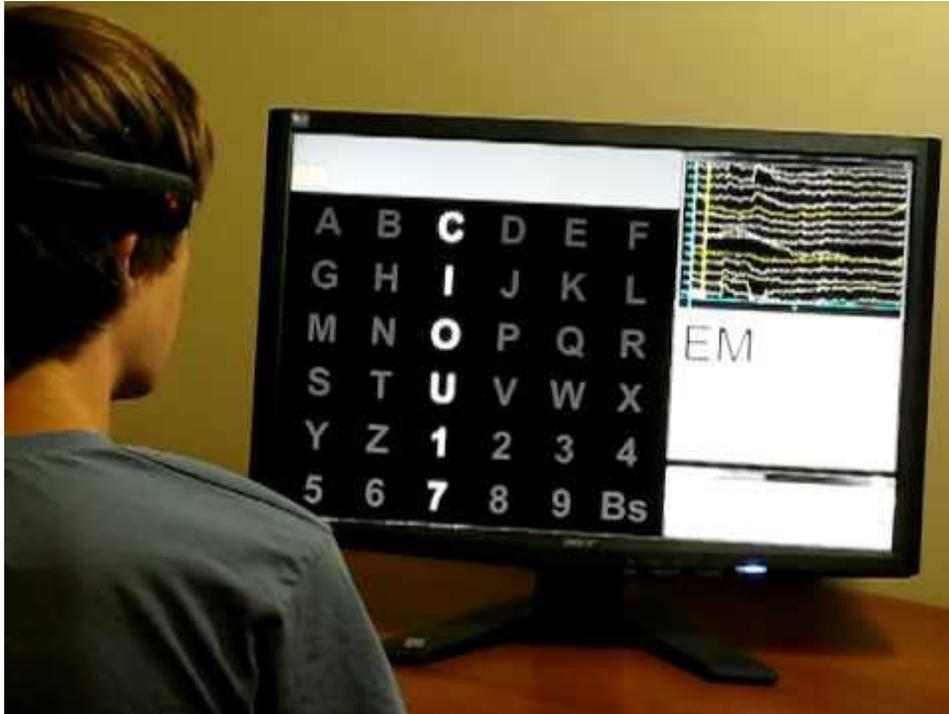
Figure 2.1: Example of a P300 type spelling BCI using a 6X6 matrix of letters, numbers, and a backspace [1]
