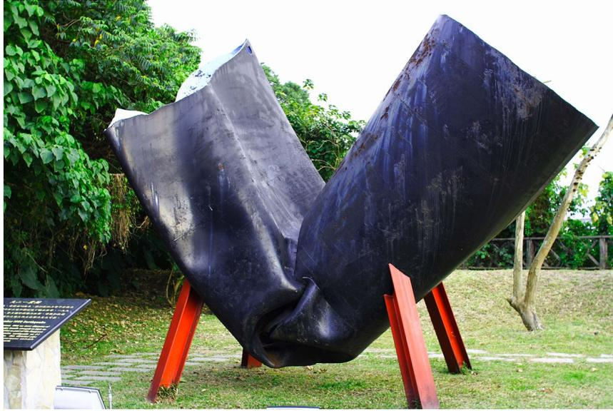
Figure 1.1: 78 inches wide and 0.7 inches thick pipe bent in Chi-Chi earthquake. [4].
