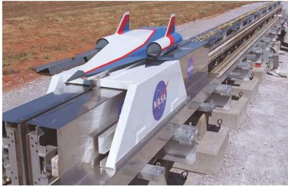
(a) Demonstration of electromagnetic launch assistance track of NASA [108].
