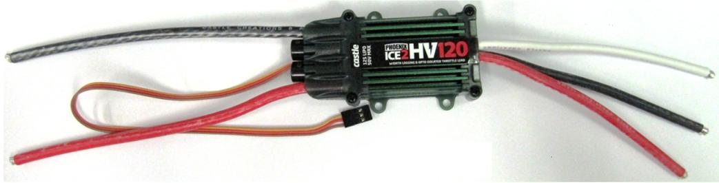
Figure 6.6: *Phoenix ICE HV 120 brushless speed controller.*
