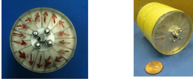
Figure 2.7 Experimental 2 pole-pair Halbach rotor with 16 segments
